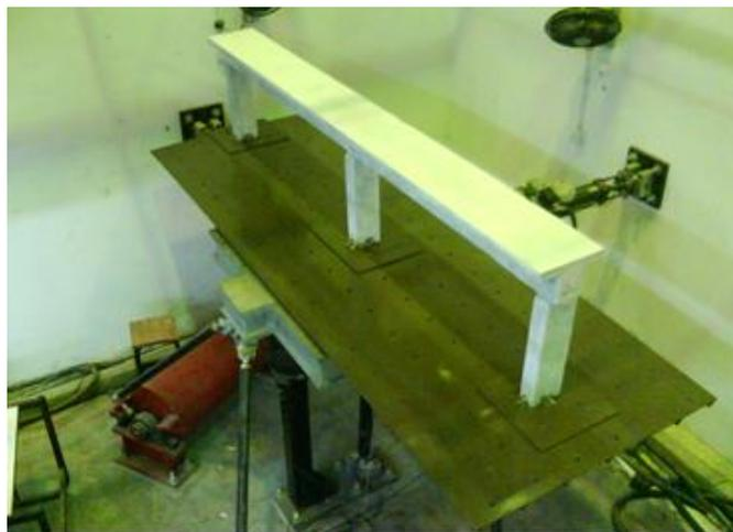
Figure 2. Table top grid of R-51 hydraulic shaking table.
