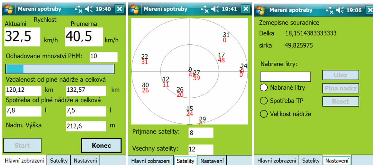
Figure 4. Screen shot examples of application (main measurement screen, satellite position, setup/refill fuel options).
