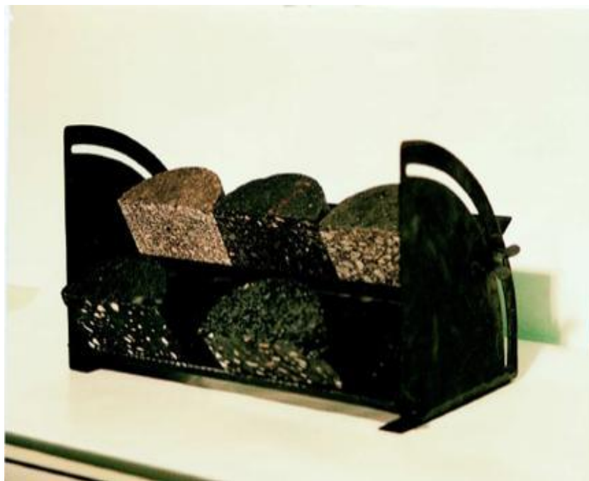
Figure 6. Equipment for testing deformation characteristics of a compacted asphaltic concrete mix on slopes.
