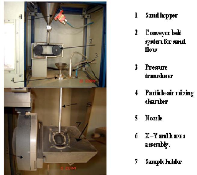
**Figure 1.** Schematic of air jet erosion test rig.
