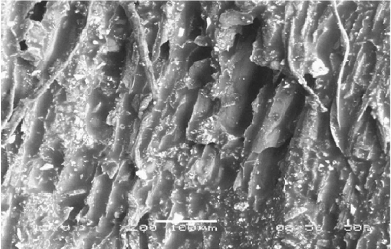
**Figure 7.** SEM micro graph of surface eroded at 30°.
