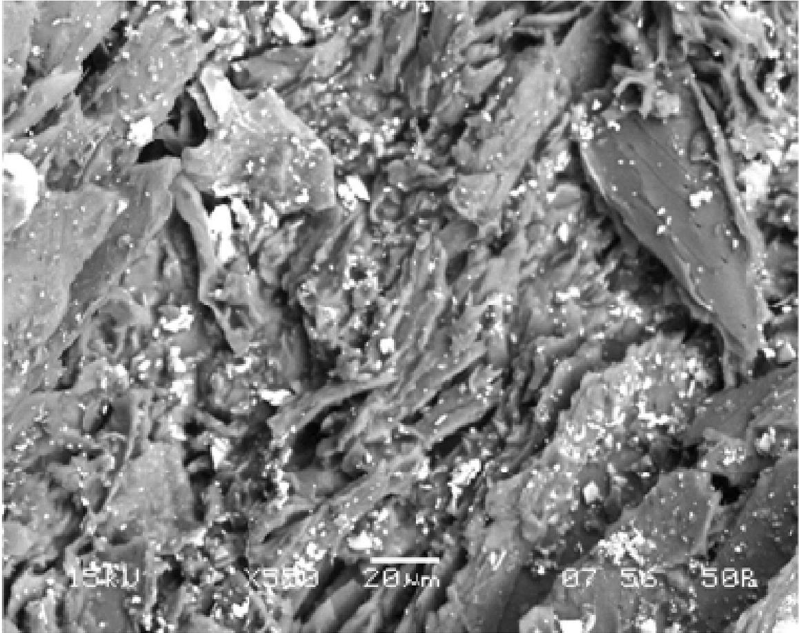
**Figure 8.** SEM micro graph of surface eroded at 45°.
