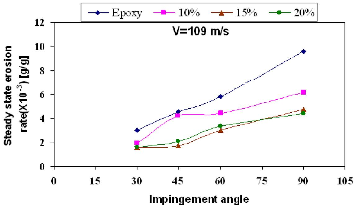
Figure 6. Variation of erosion rate as a function of angle of impingement at  $V = 109$  m/s.
