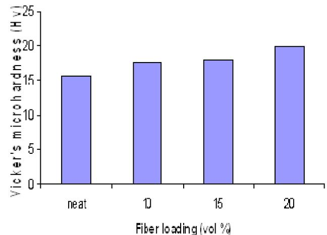
**Figure 2.** Micro hardness values for different composites.
