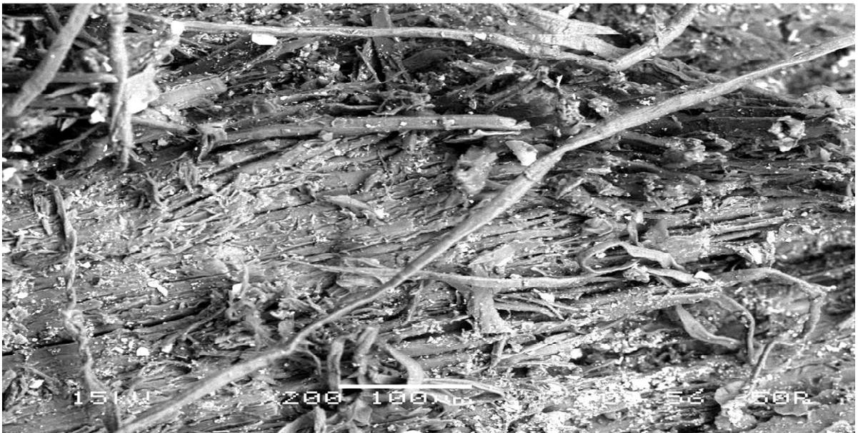
**Figure 9.** SEM micro graph of surface eroded at 60°.
