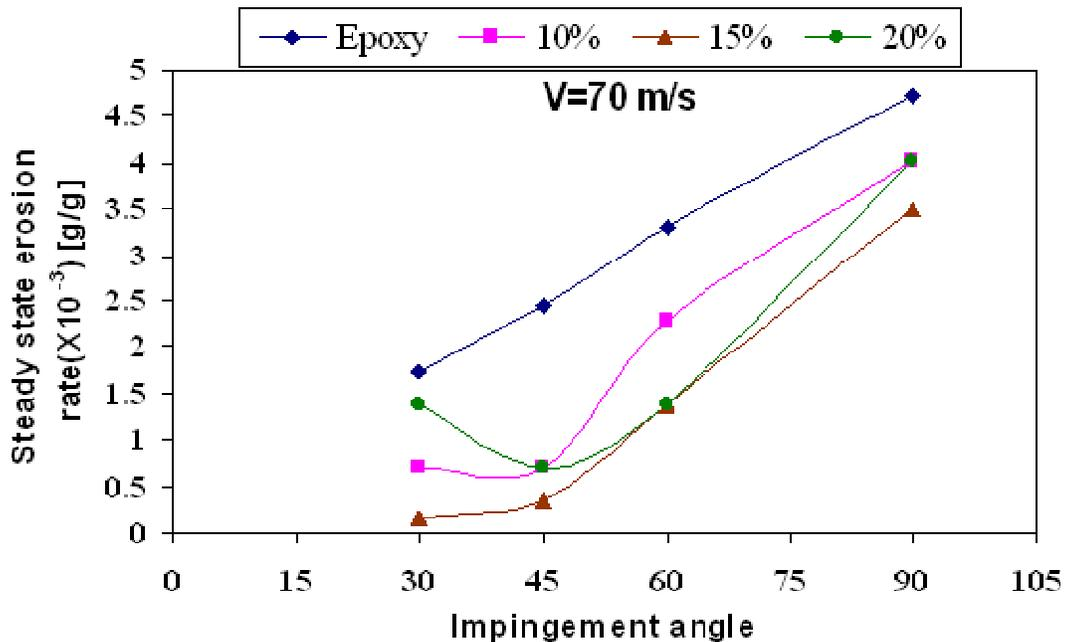
Figure 4. Variation of erosion rate as a function of angle of impingement at  $V = 70$  m/s.
