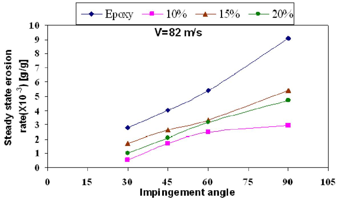
Figure 5. Variation of erosion rate as a function of angle of impingement at  $V = 82$  m/s.
