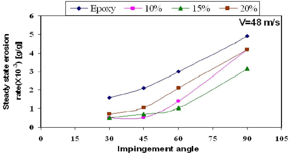
Figure 3. Variation of erosion rate as a function of angle of impingement at  $V = 48$  m/s
