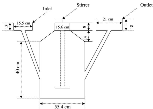
Figure 1. Schematic diagram of the biodigester.
