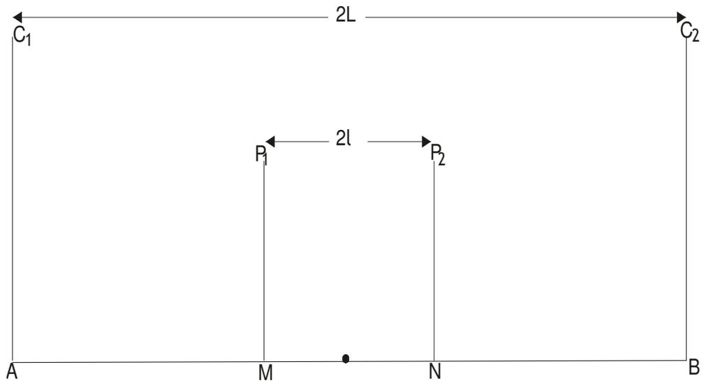
Figure 1. The Schlumberger array configuration (Whitely, 1973).
