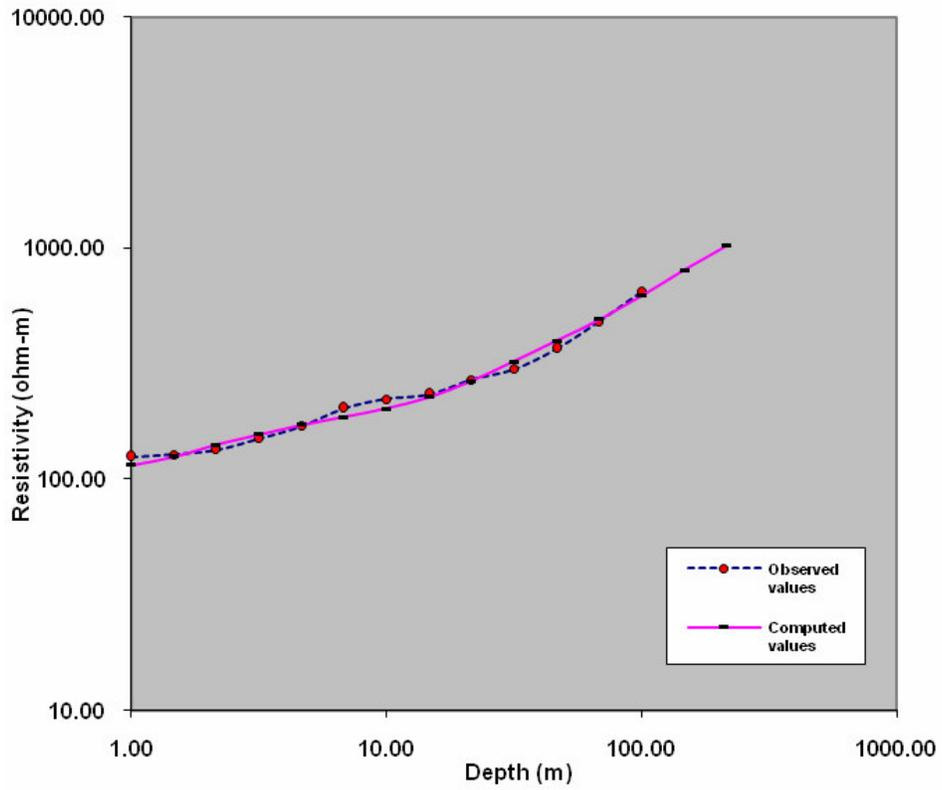
Figure 3. Field Data, theoretical curve and the layer model of New Sapele/Agbor Road Obinomba.
