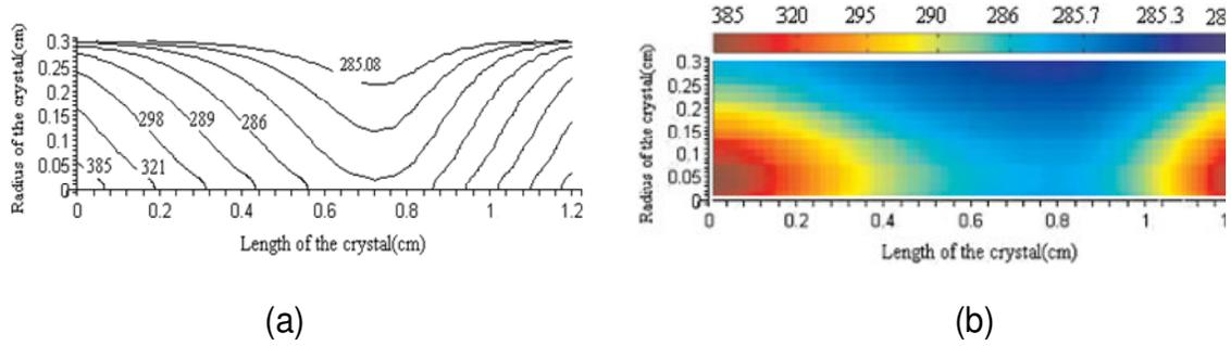
**Figure 1.** (a) The temperature distribution in the Nd:YVO<sub>4</sub> laser crystal. (b) Heat diagram in the Nd:YVO<sub>4</sub> laser crystal pumped by 10 and 5 Watts from left and right side respectively. Pumped by 10 and 5 Watts from left and right side.
