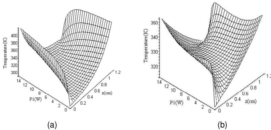
**Figure 2.** Temperature on the axis of Nd:YVO<sub>4</sub> crystal versus left pump power and distance from left surface for a = 0.2 mm. (b) Temperature on the axis of Nd:YVO<sub>4</sub> crystal versus left pump power and distance from left surface for a = 0.1 mm.
