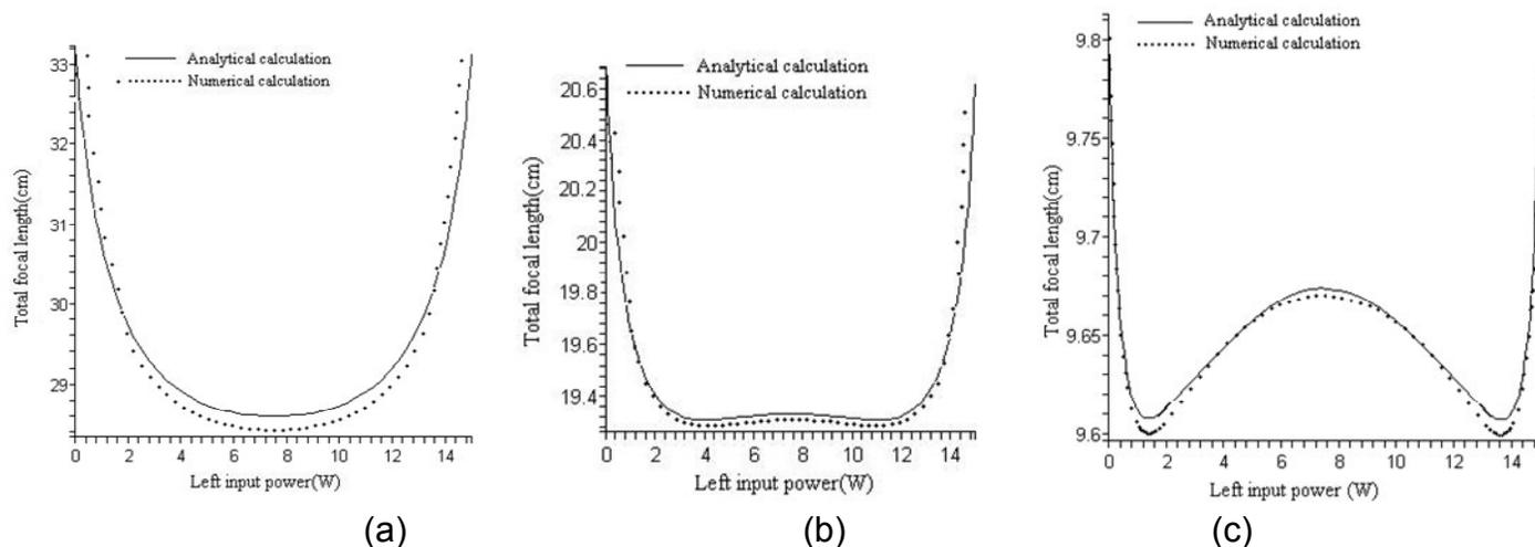
**Figure 4.** (a) Total focal length versus left versus left input power for 0.2 mm pump radius. (b) Total focal length versus left input power for 0.150 mm pump radius. (c) Total focal length input power for 0.1 mm pump radius.
