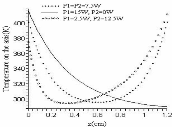
**Figure 3.** Temperature distribution versus z for three kind of pumping
