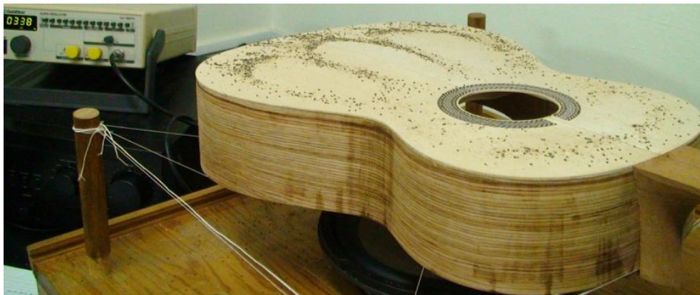
Figure 8. Obtaining the four modes on guitar vibrated in the final stages of manufacturing.
