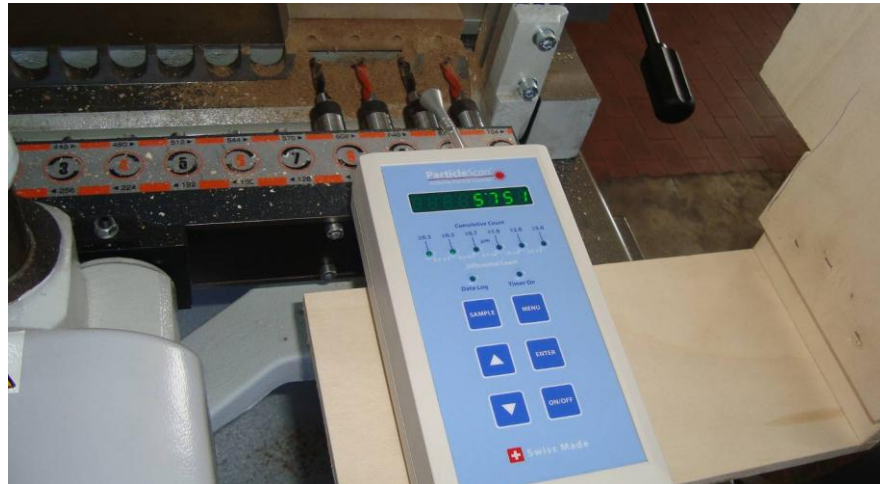
Figure 1. Placement of the particle measuring instrument closer to the source of particles, avoiding the environmental impacts.
