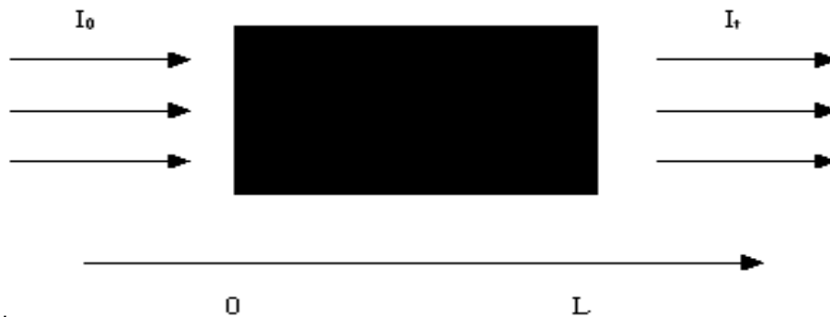
Figure 9. Penetration of a truss of parallel radiation into water fog screen.
