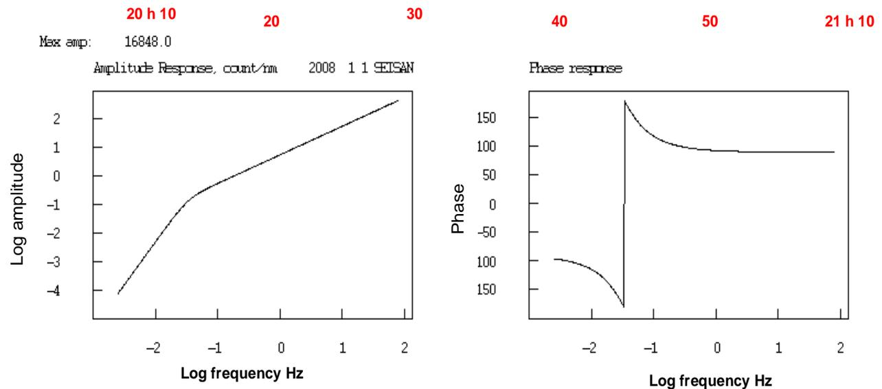
Figure 10. Amplitude and phase responses from Nsukka Station (Z-component).
