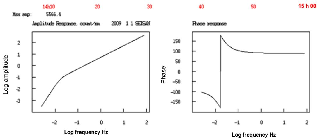
Figure 8. Amplitude and phase responses from Kaduna Station (Z-component).
