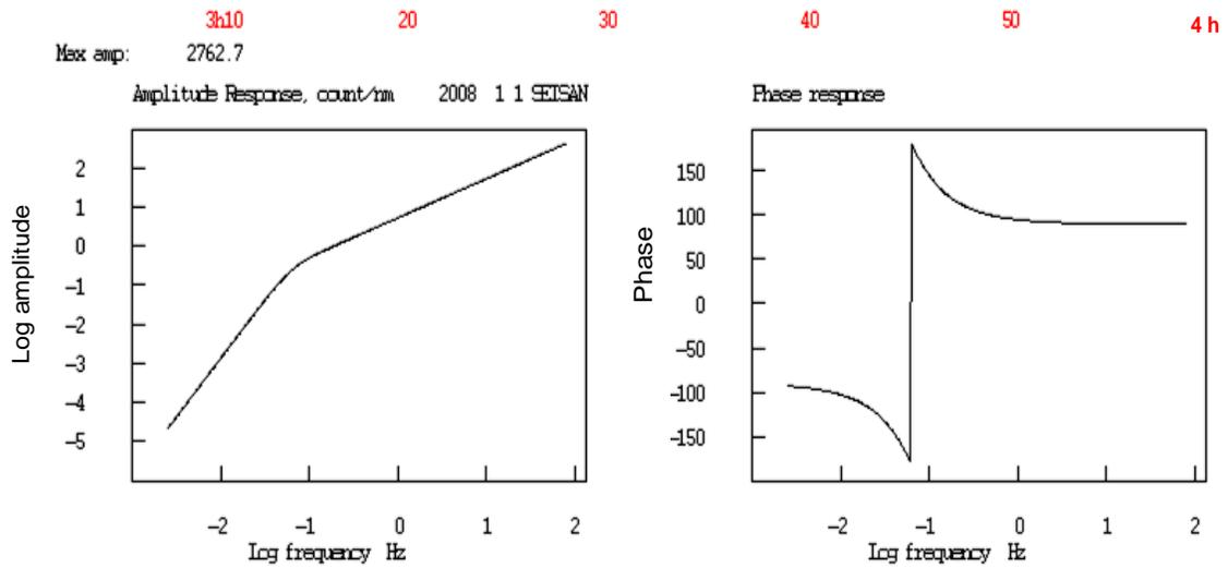
Figure 6. Amplitude and phase responses from Ife Station (Z-component).
