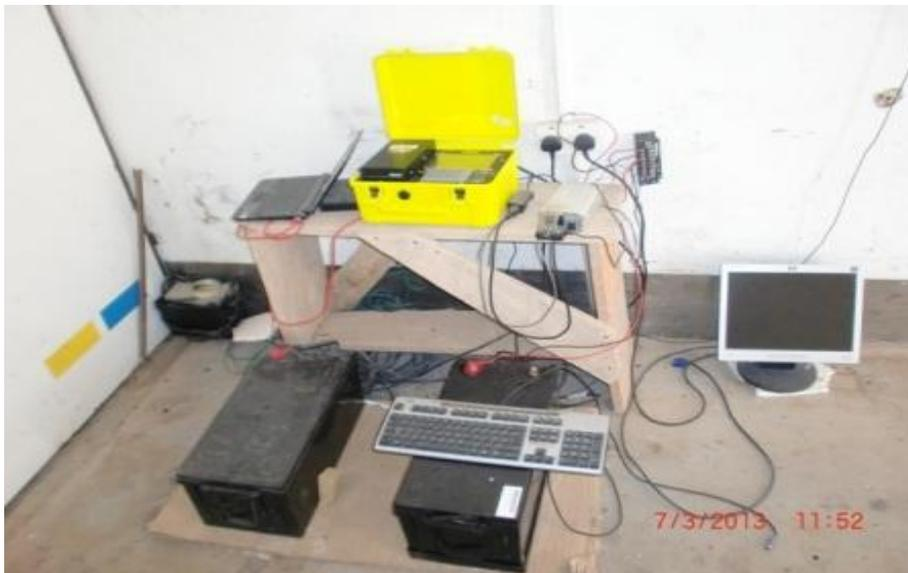
**Figure 4.** A typical set up of NNSS stations; this one at Toro station showing recorder, batteries connected to solar panels installed outside, computer monitor to temporary store data before they are downloaded and processed.
