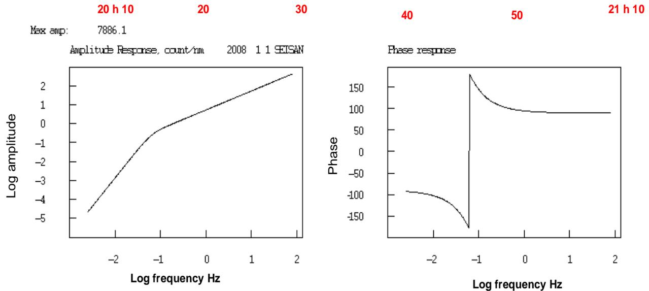
Figure 9. Amplitude and phase responses from Nsukka Station (Z-Component).
