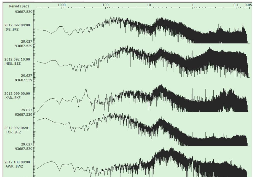
**Figure 12.** Noise spectra of (from top Ife, Nsukka, Kaduna, Toro and Awka). The spectra were here not compared with Peterson (1993) noise models.
