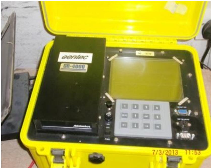
**Figure 3.** A DR 4000 Eentec recorder at Toro Station.
