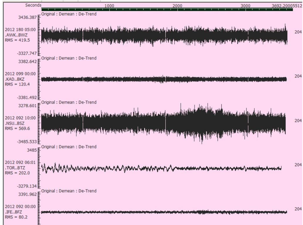
**Figure 11.** Showing noise traces (from top: Awka, Kaduna, Nsukka, Toro and Ife). No filters were applied, but the mean and other trends were removed.
