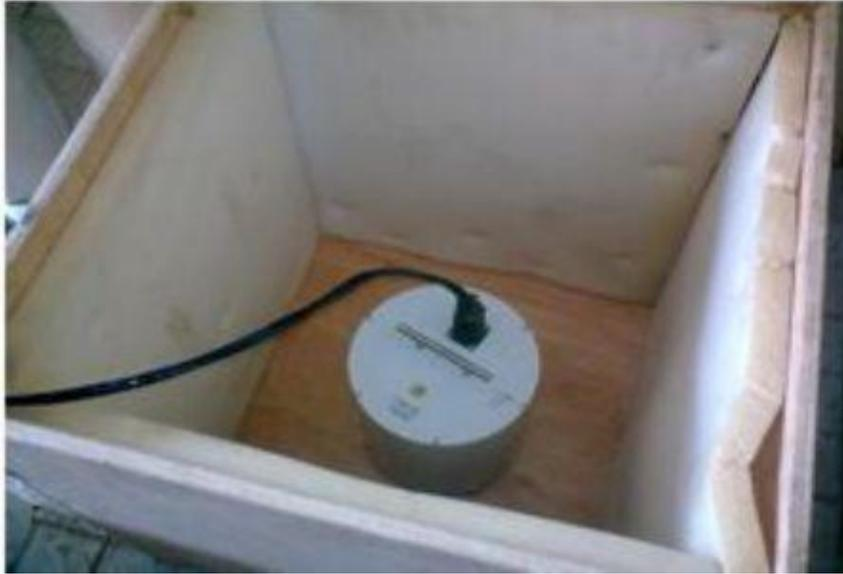
**Figure 2.** A Eentec EP 105 sensor installed and insulated at Toro Station.
