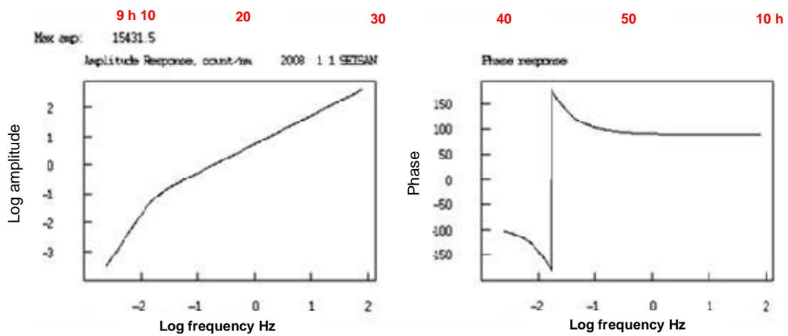
Figure 7. Amplitude and phase responses from Toro Station (Z-component).
