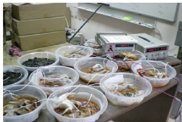
Figure 3. The first series of 10 groups subjected to corrosion under cathodic protection.
