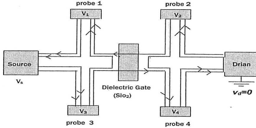
**Figure. 6.** A quantitative picture of double-gate with four voltage probe (Bahari et al., 2009).
