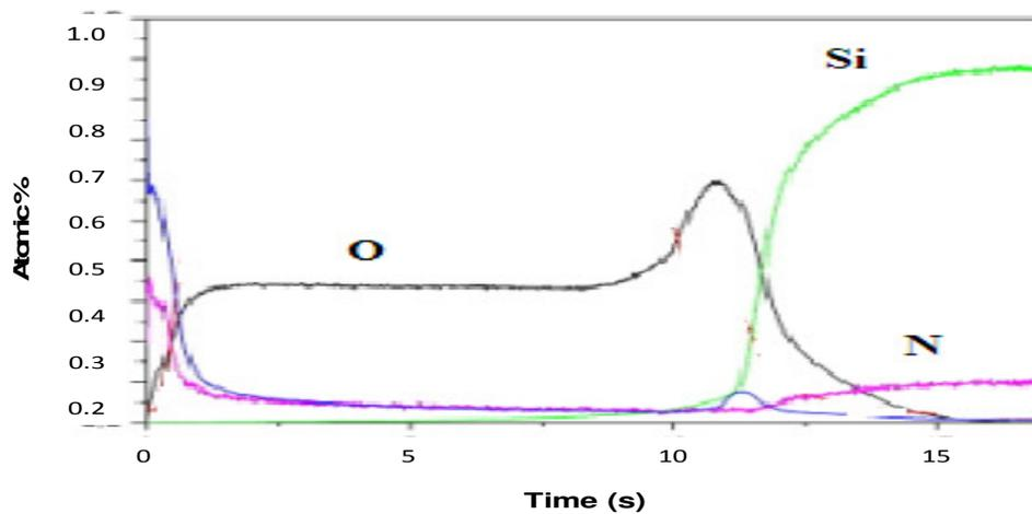
Figure 2. Sputtering profile of silicon oxynitride.
