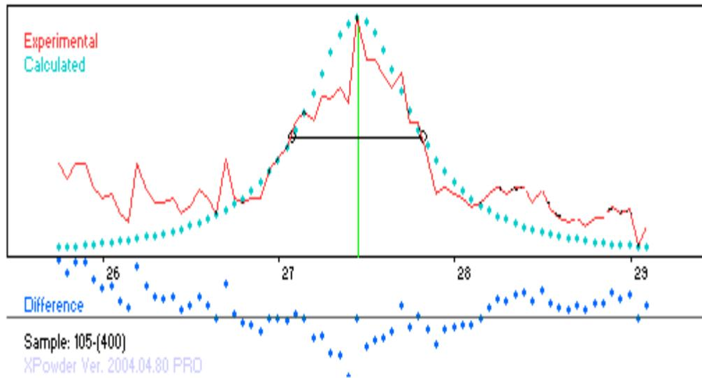
**Figure 5.** As an example, the correction of determination of a particle size into the film. Dashed line below the background line shows the difference from experimental and calculated data.
