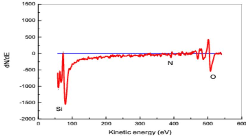
Figure 1. AES spectrum of silicon nitride.
