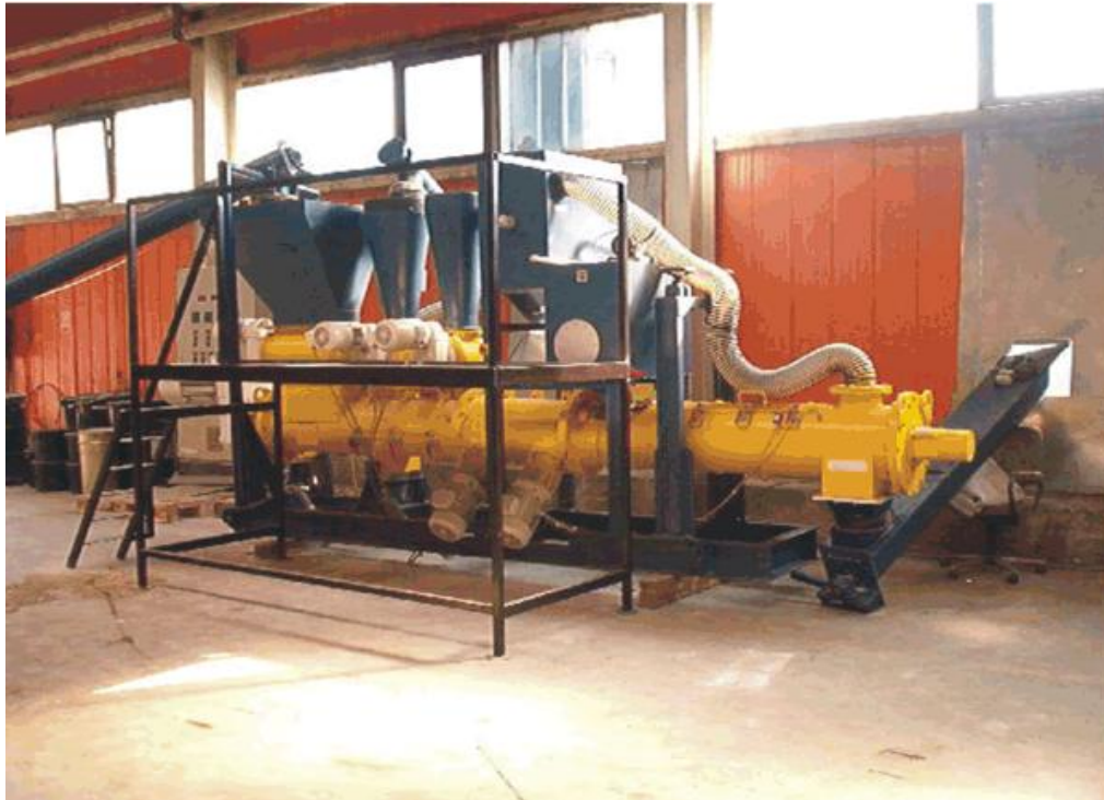
Figure 3. General look of the MID-MIX® mobile plant with capacity of 10 m 3 /h for treatment of different sorts of cobble hydrogenised waste placed in the hall (Maribor – Slovenia 2000), (www.grgoni.hr, 2011).
