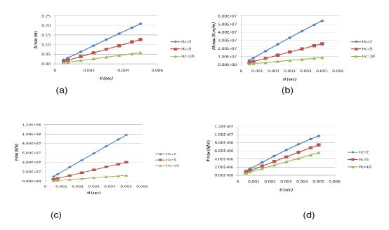
Figure 10. (a) Maximum roof deflections, (b) Maximum roof moments, (c) Maximum roof shear force and (d) Maximum roof axial force vs. impulse duration for variation of burial depth.
