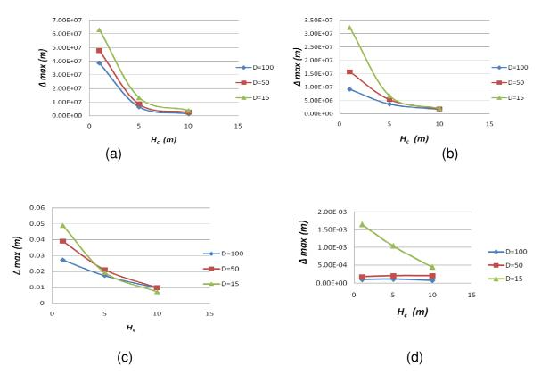
Figure 11. (a) Maximum roof shear force, (b) Maximum roof moment, (c) Maximum roof deflection and (d) Maximum wall deflections vs. burial depth for variation of tank diameter
