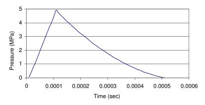
Figure 2. Typical load time history in near field explosion.
