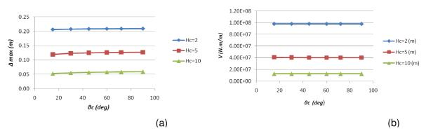
Figure 6. (a) Maximum roof deflections and (b) Maximum internal roof shear forces vs. column alignment factors.
