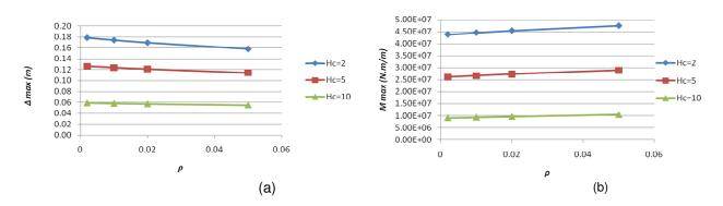
Figure 4. (a) Maximum roof deflections and (b) Maximum roof moments vs. burial depth for variation of steel ratio.
