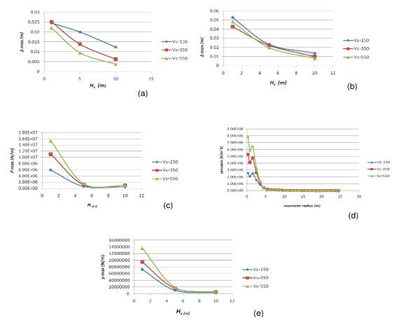
**Figure 9.** (a) Maximum bottom deflection, (b) Maximum roof deflection, (c) Maximum roof axial force, (d) Maximum central column axial force and (e) impulsive overpressure distribution on roof vs. burial depth for various soil elastic modulus (Here  $V_s$  is the shear wave velocity in soil and represents the variation of soil elastic modulus).
