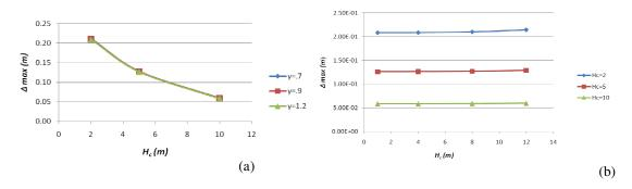
Figure 5. (a) Maximum roof deflections and (b) Maximum roof moments vs. burial depth for variation of steel ratio.
