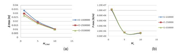
Figure 8. (a) Maximum roof deflections and (b) Maximum roof axial force vs. burial depth for variation of concrete elastic modulus.
