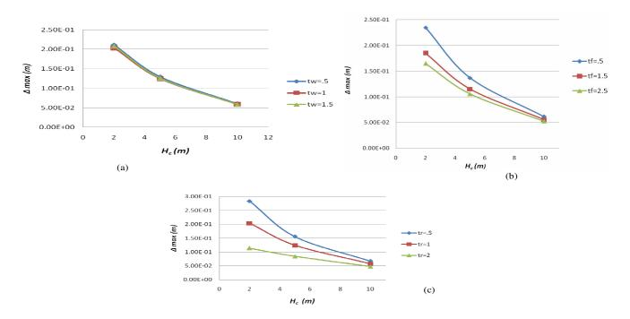
Figure 3. Maximum roof deflections vs. burial depth for (a) wall thickness, (b) bottom thickness and (c) roof thickness variation.
