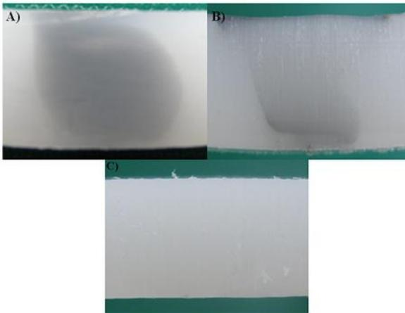
**Figure 5.** Macroscopic sections that illustrated material degradation in various shoulder temperature: (a) the material at stir zone is degraded in test 1, (b) material degradation occurred only in bottom of welding zone in test 2 and (c) a sound weld without any degradation in test 3.
