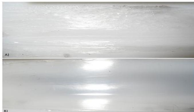
**Figure 8.** Effect of tool shoulder coating on surface quality of welded polyethylene sheets: (a) welding by shoulder without coating and (b) welding by coated shoulder.
