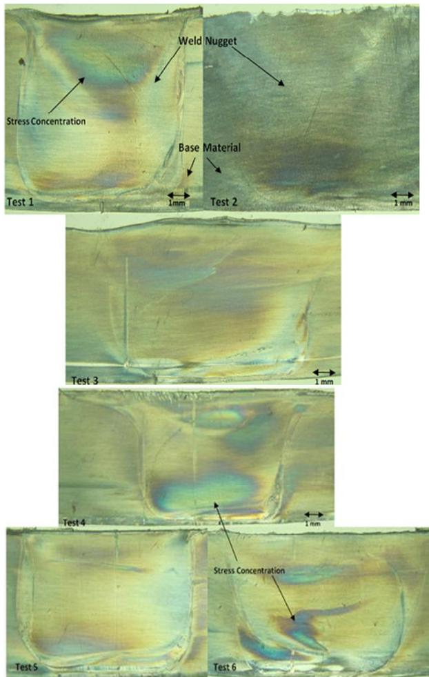
**Figure 6.** Microstructure observations of weld sections obtained from photolastic polarscope device.
