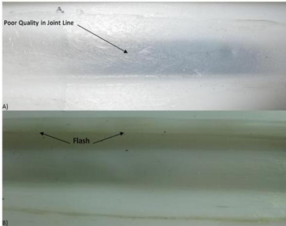
**Figure 4.** Effect of tool plunge depth on joint surface quality: (a) lower plunge depth and (b) higher plunge depth.
