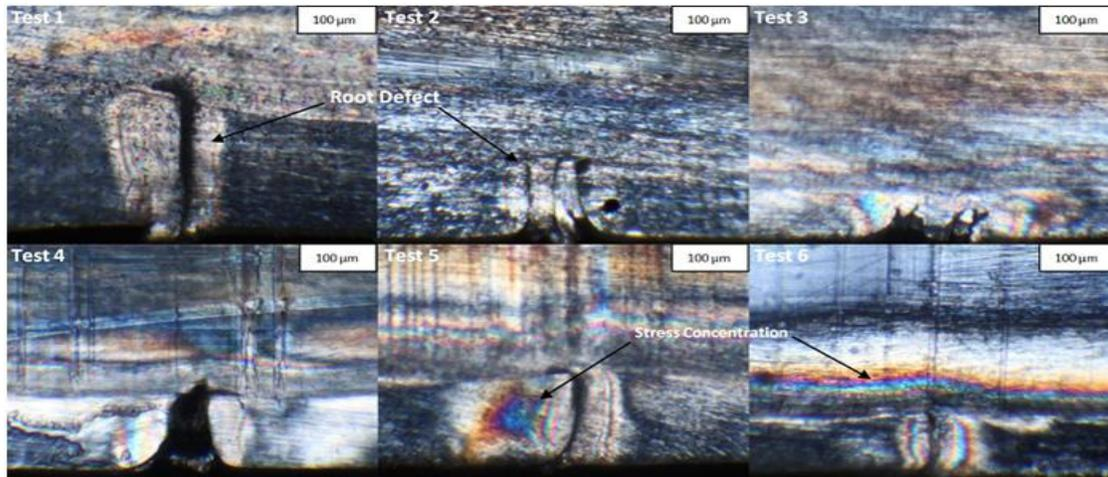
**Figure 7.** Root penetration defect of various test condition.
