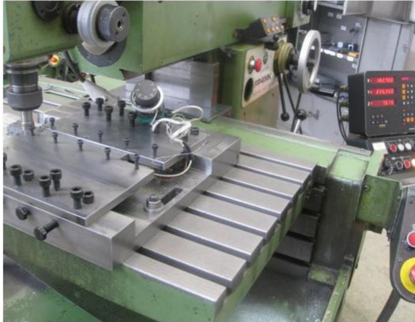
**Figure 2.** Heat assisted friction stir welding of HDPE sheets.
