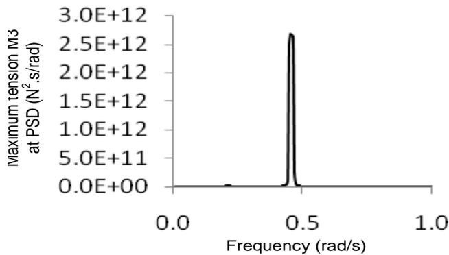
**Figure 20.** Maximum tension at Mooring line 3 at PSD after 10000 s of wave hitting.
