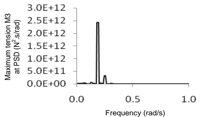
**Figure 18.** Maximum tension at Mooring line 3 at PSD after 3000 s of wave hitting.
