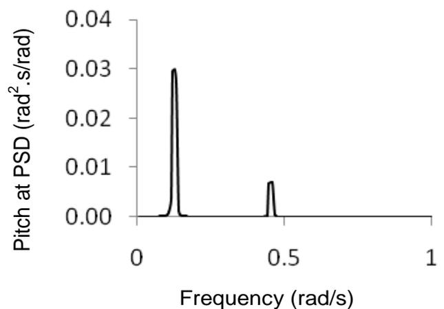
Figure 12. Pitch response at PSD after 10000 s of wave hitting.
