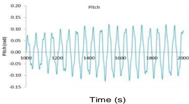
Figure 9. Pitch time series after 1000 s of wave hitting.
