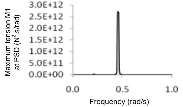
**Figure 16.** Maximum tension at Mooring line 1 at PSD after 10000 s of wave hitting.
