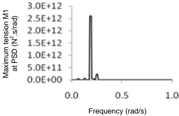
**Figure 14.** Maximum tension at Mooring line 1 at PSD after 3000 s of wave hitting.
