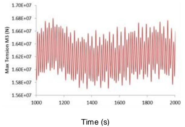
**Figure 17.** Maximum tension time series of Mooring line 3 after 1000 s of wave hitting.
