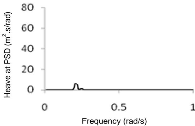
Figure 8. Heave response at PSD after 10000 s of wave hitting.
