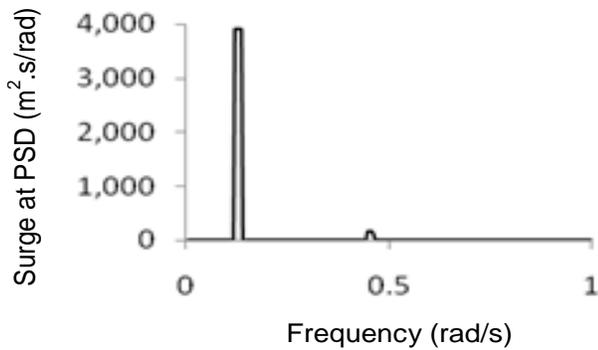
Figure 2. Surge response at PSD after 3000 s of wave hitting.
