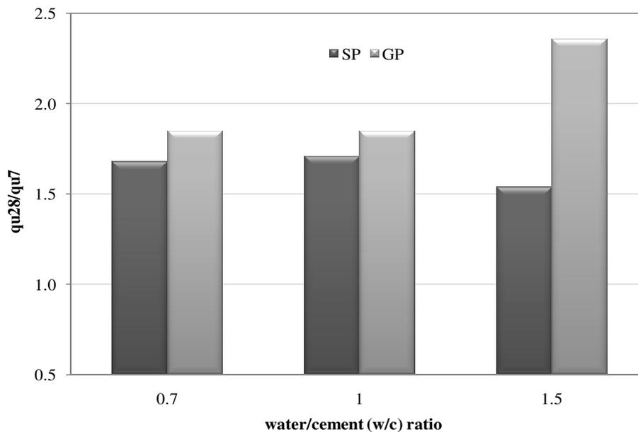
**Figure 6.** Variation of unconfined compressive strength of 28 and 7-day-cured specimens (denoted as  $q_{u28}$  and  $q_{u7}$ ) with water/cement ratio.
