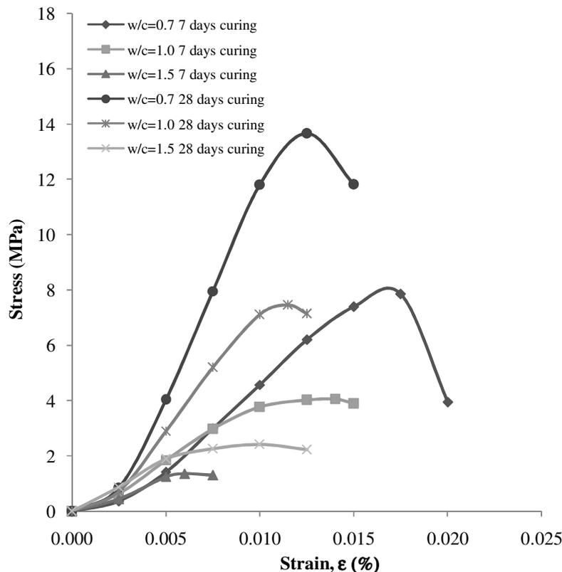
**Figure 3b.** Unconfined compression strengths of SP sample ( $D_r = 75\%$  and  $P = 150$  kPa).
