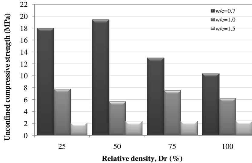
**Figure 5b.** Variation of the unconfined compressive strength with relative density for SP samples.
