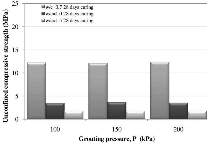
**Figure 4a.** Variation of unconfined compressive strength with grouting pressure for GP sample with  $D_r = 50\%$ .
