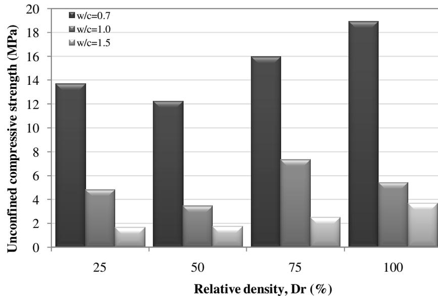
**Figure 5a.** Variation of unconfined compressive strength with relative density for GP samples.
