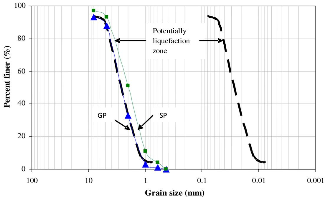
**Figure 1.** Particle size distribution of test samples.**Table 2.** Basic properties of the soil samples.
