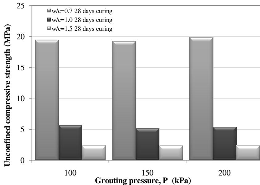
**Figure 4b.** Variation of unconfined compressive strength with grouting pressure of SP sample with  $D_r = 50\%$ .
