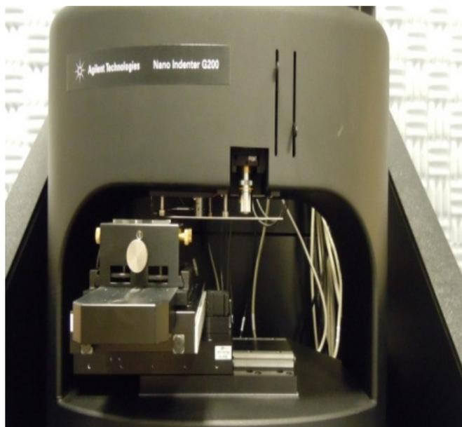
**Figure 1.** Nano Indenter G200.**Table 2.** Nano Indenter G200 Specifications.
