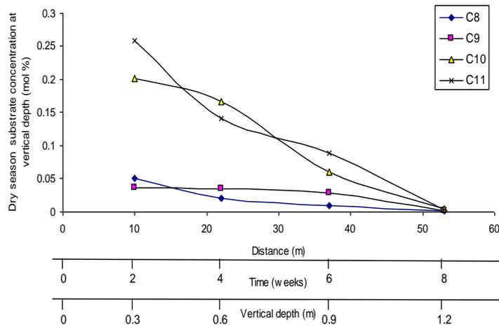
**Figure 8.** Dry season substrate concentration at vertical direction versus distance, time, and vertical depth (for B<sub>1</sub>).
