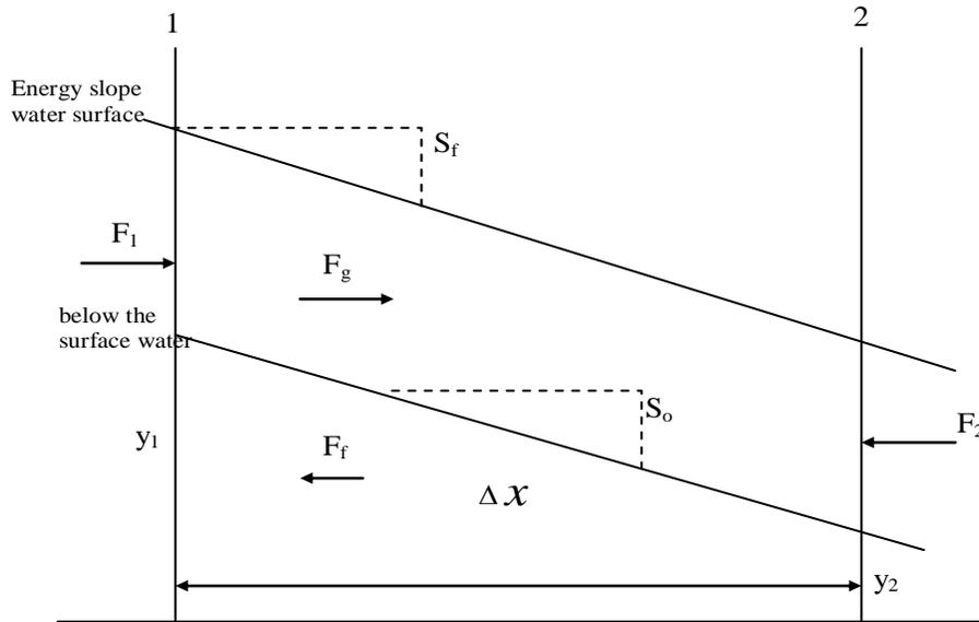
Figure 1. Force balance on a fluid element in a pond.
