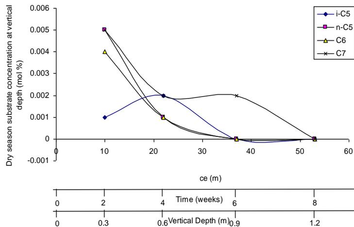
**Figure 13.** Dry season substrate concentration at vertical direction versus distance, time, and vertical depth (for B<sub>4</sub>).
