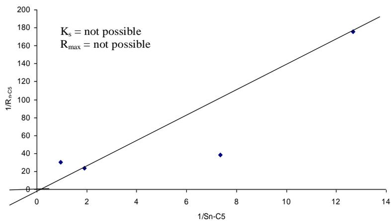
**Figure 16.** Dry season line weaver bulk plot for  $1/R_{n-C5}$  versus  $1/S_{n-C5}$ .
