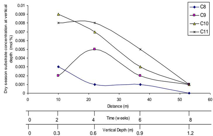
**Figure 14.** Dry season substrate concentration at vertical direction versus distance, time, and vertical depth (for B<sub>4</sub>).
