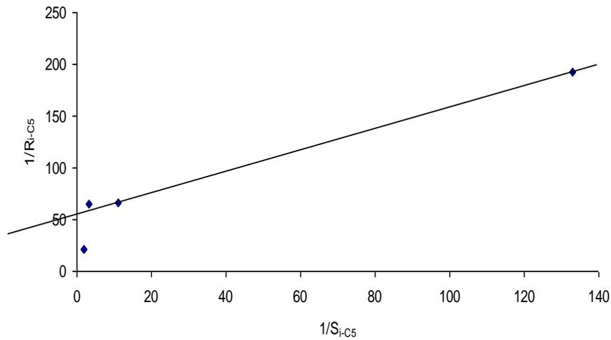
**Figure 15.** Dry season line weaver bulk plot for  $1/R_{i-C5}$  versus  $1/S_{i-C5}$ .
