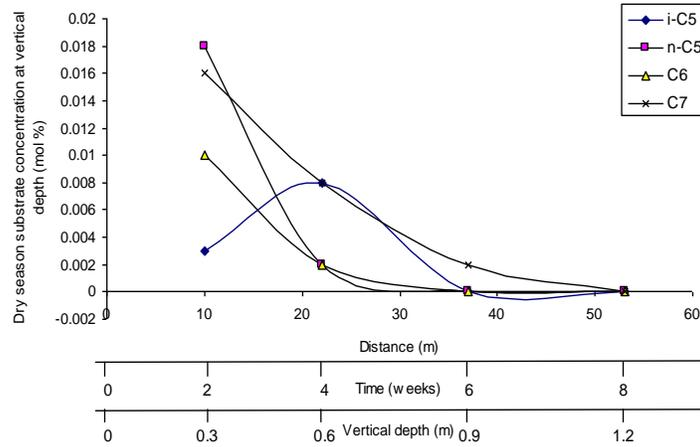
**Figure 11.** Dry season substrate concentration at vertical direction versus distance, time, and vertical depth (for B<sub>3</sub>).
