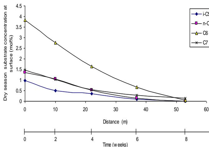
**Figure 3.** Dry season substrate concentration at surface versus distance and time.
