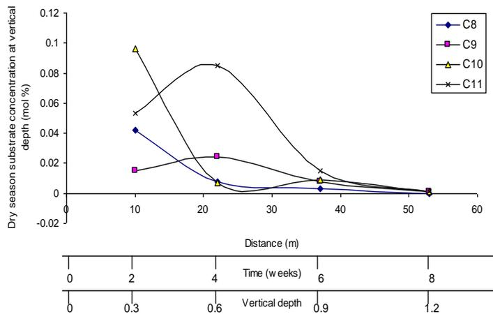
**Figure 10.** Dry season substrate concentration at vertical direction versus distance, time, and vertical depth (for B<sub>2</sub>).
