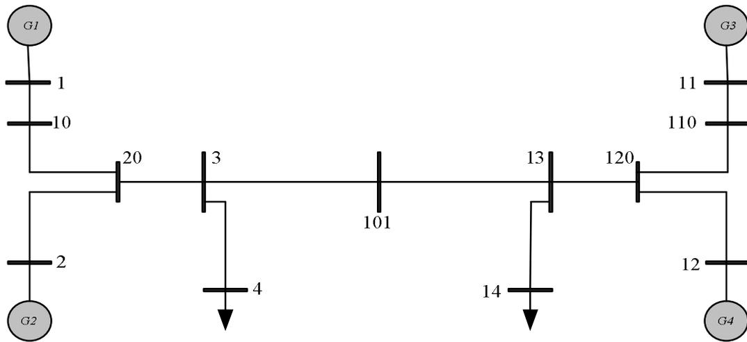
Figure 3. Single line diagram of 2-area four machine test system.
