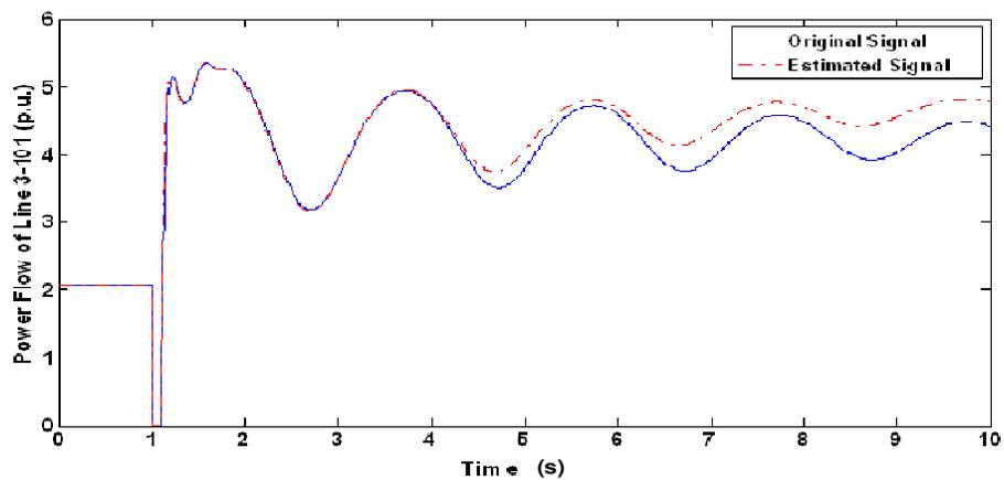
Figure 4. Measured tie line power and estimated signal.
