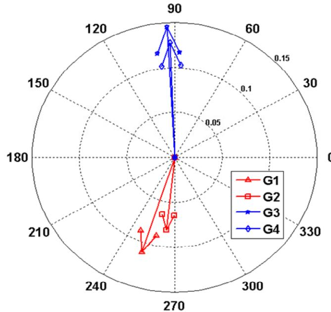
**Figure 5.** Amplitude and phase of 20th mode oscillations in generators' rotors.
