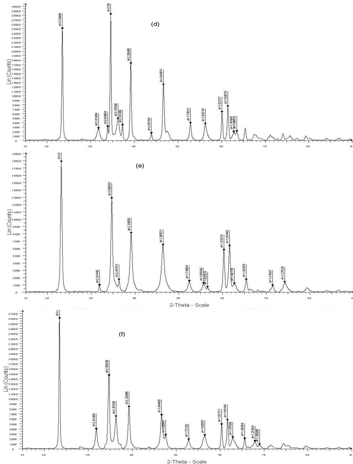
**Figure 2.** PXRD patterns obtained for HT's. (a) PXRD pattern obtained for  $Mg_4Al_2(OH)_{12}CO_3 \cdot 3H_2O$ , (b) PXRD pattern obtained for  $Mg_6Al_2(OH)_{16}CO_3 \cdot 4H_2O$ , (c) PXRD pattern obtained for  $Zn_4Al_2(OH)_{12}CO_3 \cdot 3H_2O$ , (d) PXRD pattern obtained for  $Zn_6Al_2(OH)_{16}CO_3 \cdot 4H_2O$ , (e) PXRD pattern obtained for  $Mg_4Zn_2Al_2(OH)_{12}CO_3 \cdot 3H_2O$ , (f) PXRD pattern obtained for  $Mg_2Zn_4Al_2(OH)_{12}CO_3 \cdot 3H_2O$ .
