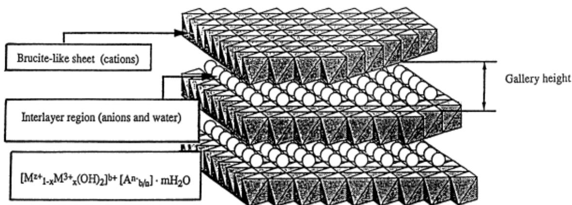
**Figure 1.** Layered structure of hydrotalcites with rhombohedral symmetry.
