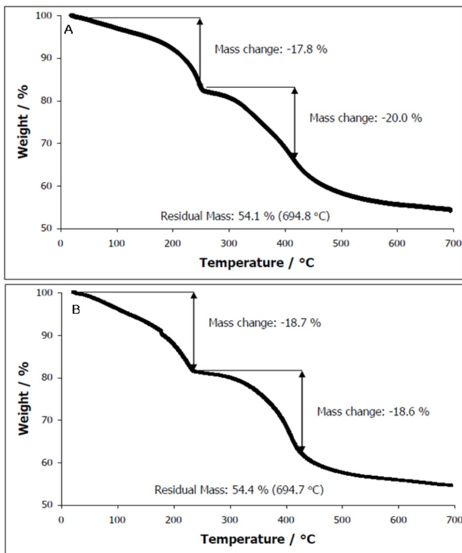
**Figure 3.** Thermograms for (A) Mg<sub>4</sub>Al<sub>2</sub>-HT and (B) Mg<sub>6</sub>Al<sub>2</sub>-HT.
