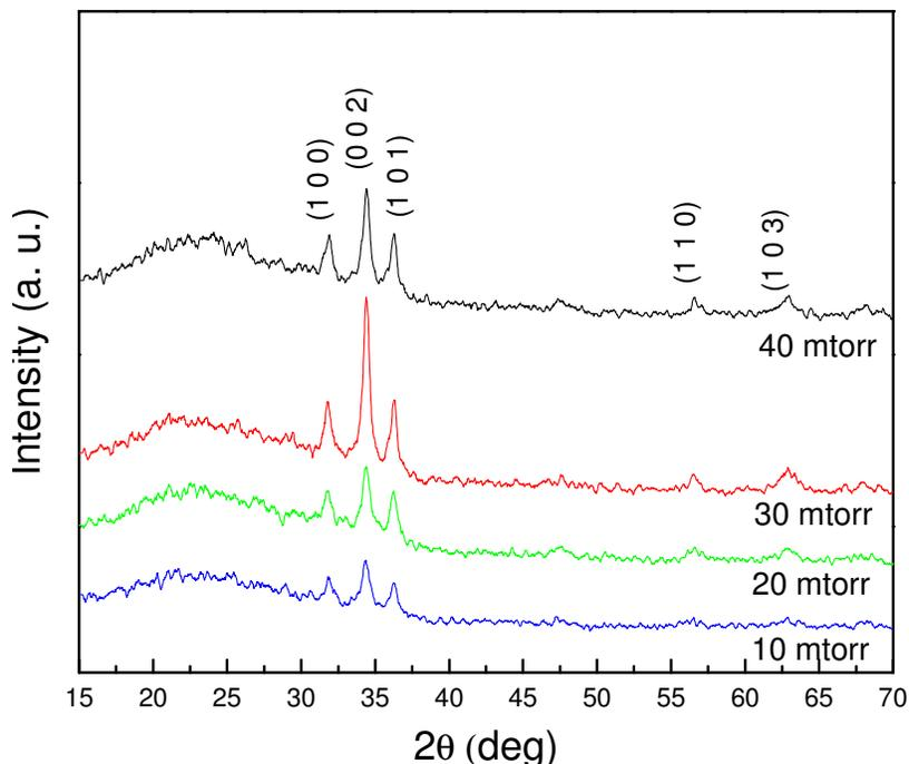
**Figure 2.** XRD peaks for  $\text{ZnO}_{1-\delta}$  films grown at  $300^\circ\text{C}$  under different  $\text{PO}_2$ .
