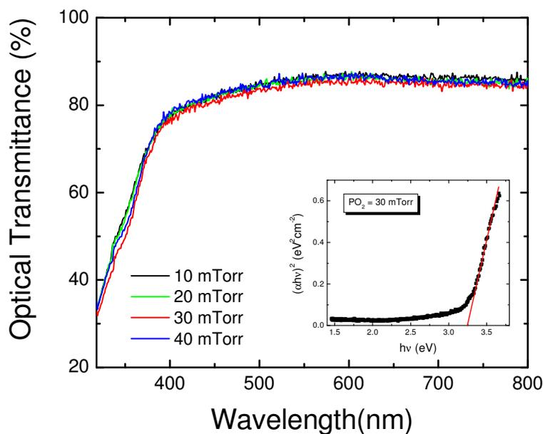
Figure 4. Optical transmittance spectra of ZnO<sub>1-δ</sub> films under different PO<sub>2</sub>.
