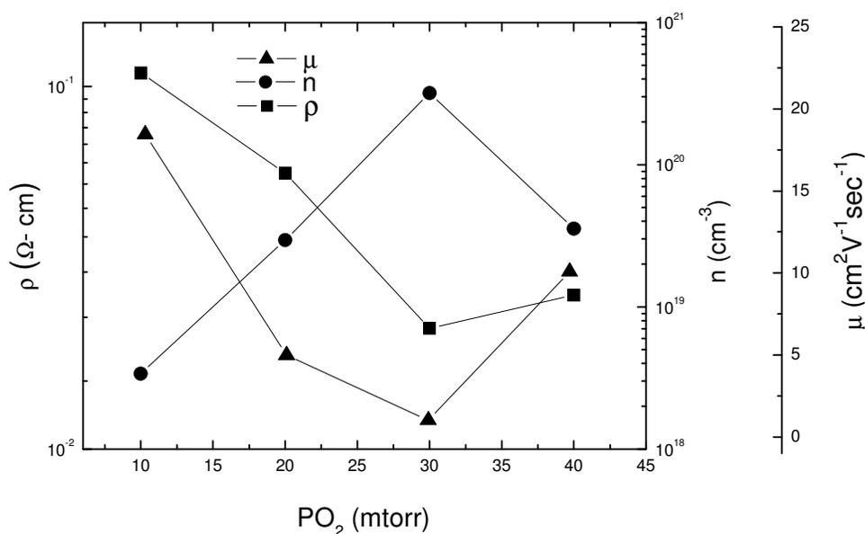
**Figure 1.** Variations in resistivity, carrier concentration, and carrier mobility as functions of oxygen pressure for ZnO<sub>1-δ</sub> deposited at deposition temperature of 300°C.
