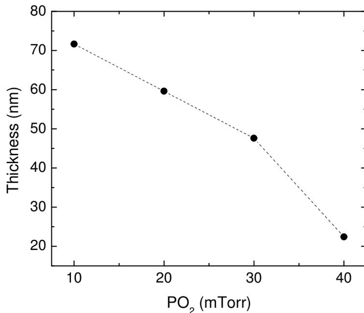
Figure 3. Thickness for the PLD ZnO<sub>1-δ</sub> films as a function of the PO<sub>2</sub>.
