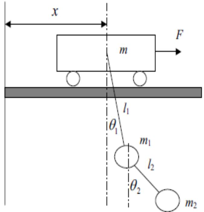
**Figure 1.** Model of a double-pendulum-type overhead crane.
