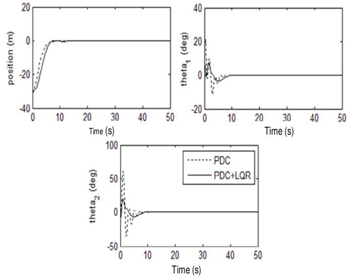
Figure 2. System dynamics of the overhead crane with PDC and parallel distributed fuzzy LQR controller.
