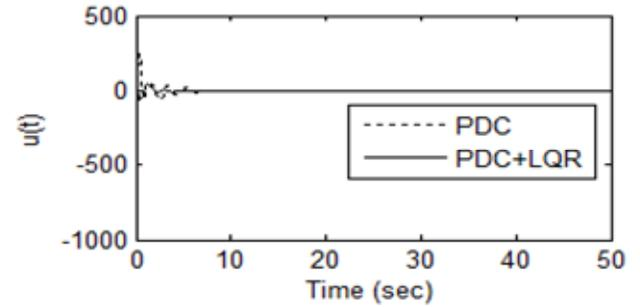
Figure 3. Control signals of PDC and parallel distributed fuzzy LQR controller.
