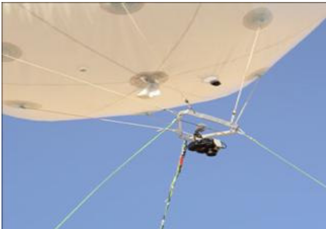
Figure 2. Balloon and camera platform (Altan et al., 2004).
