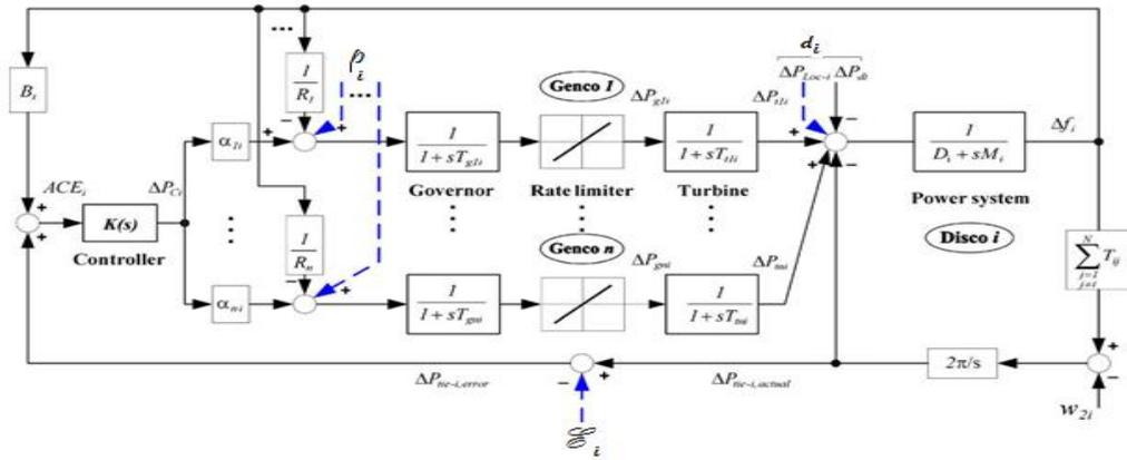
Figure 2. Control structure with GRC for ith area.
