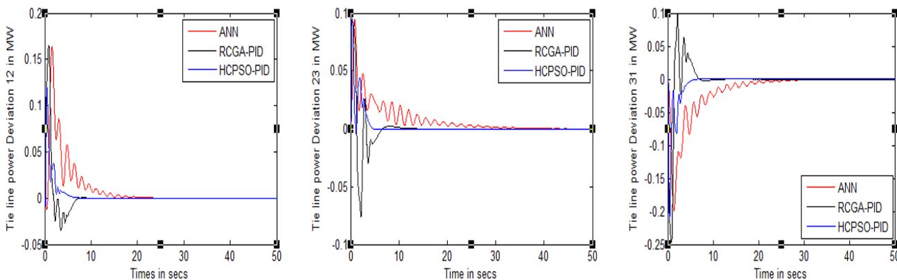
Figure 6. Tie line power deviation for scenario 1.
