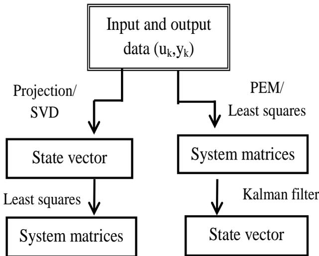
Figure 1. Subspace and PEM methods in system identification.
