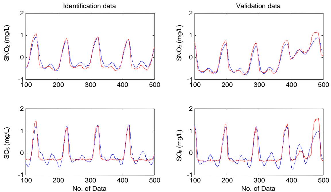
Figure 9. Identification and validation data for dry influent with 'robust' N4SID.
