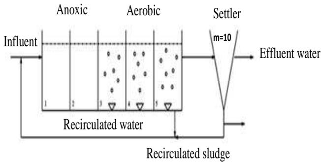
Figure 3. The Plant Layout of the BSM1.
