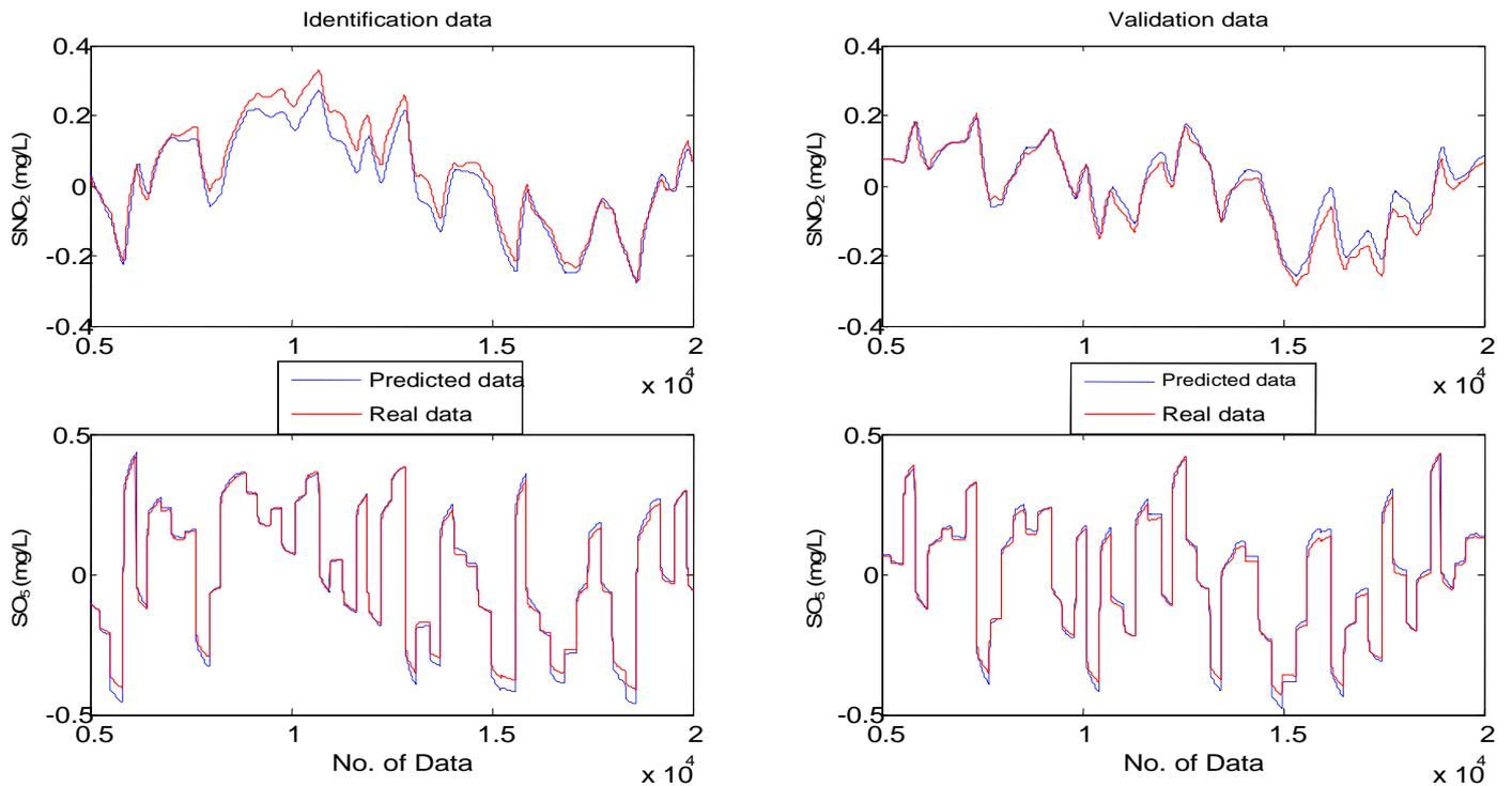
Figure 8. Identification and validation data for constant influent with 'robust' N4SID.
