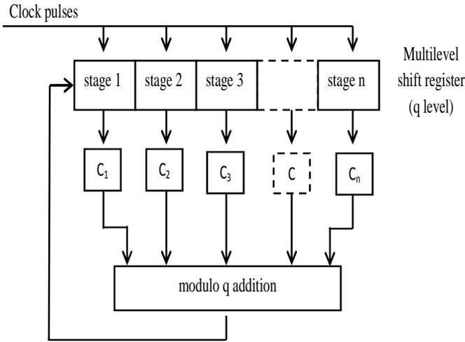
**Figure 2.** A generator of a  $q$ -level pseudo random binary sequence using shift register and modulo  $q$  addition.
