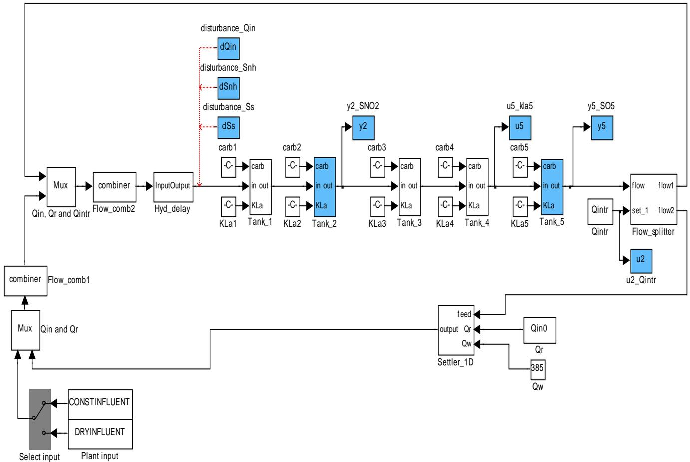
Figure 4. Signals for state-space identification.
