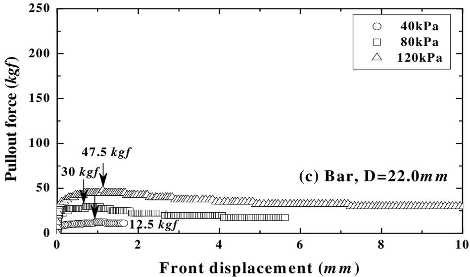
Figure 5. Front displacement-pullout force relationships for various types of steel reinforcement.
