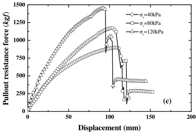
Figure 7. Relationship between displacement and pullout resistance force through laboratory tests: (a) Chain, (b) Chain with L-type angle and (c) Chain with L-type angle and transverse steel bar.
