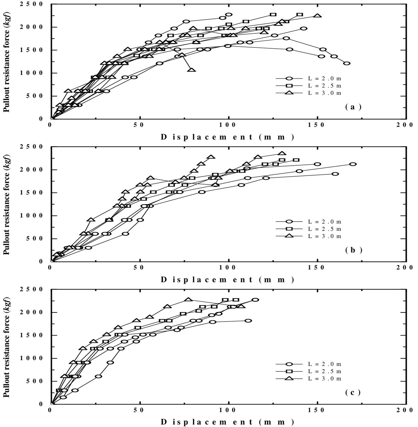
Figure 9. Relationship between displacement and pullout resistance force through *in-situ* tests: (a) Chain, (b) Chain with transverse steel bar and (c) Chain with L-type angle.
