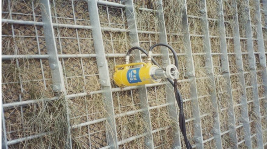
**Photo 3.** Pullout test setup using hollow cylinder.
