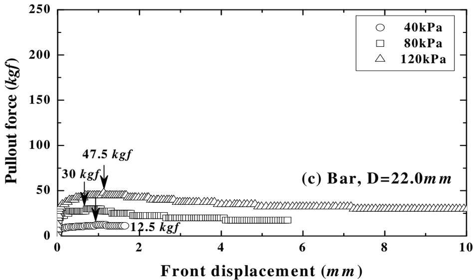
Figure 5. Front displacement-pullout force relationships for various types of steel reinforcement.
