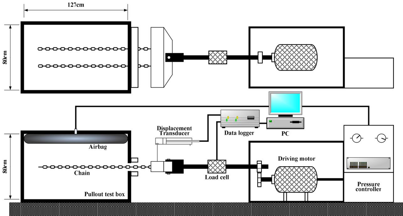
Figure 3. A Schematic diagram of laboratory pullout test equipment.
