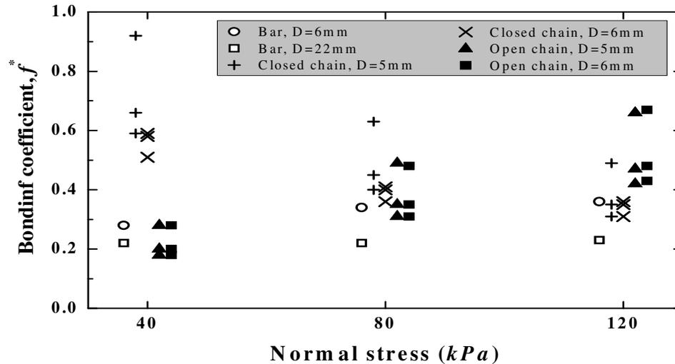
Figure 6. Bonding coefficients for various types of steel reinforcement.
