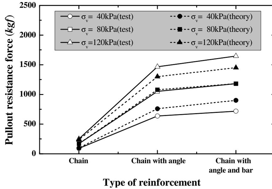
Figure 8. Pullout resistance force with variation in type of reinforcement.
