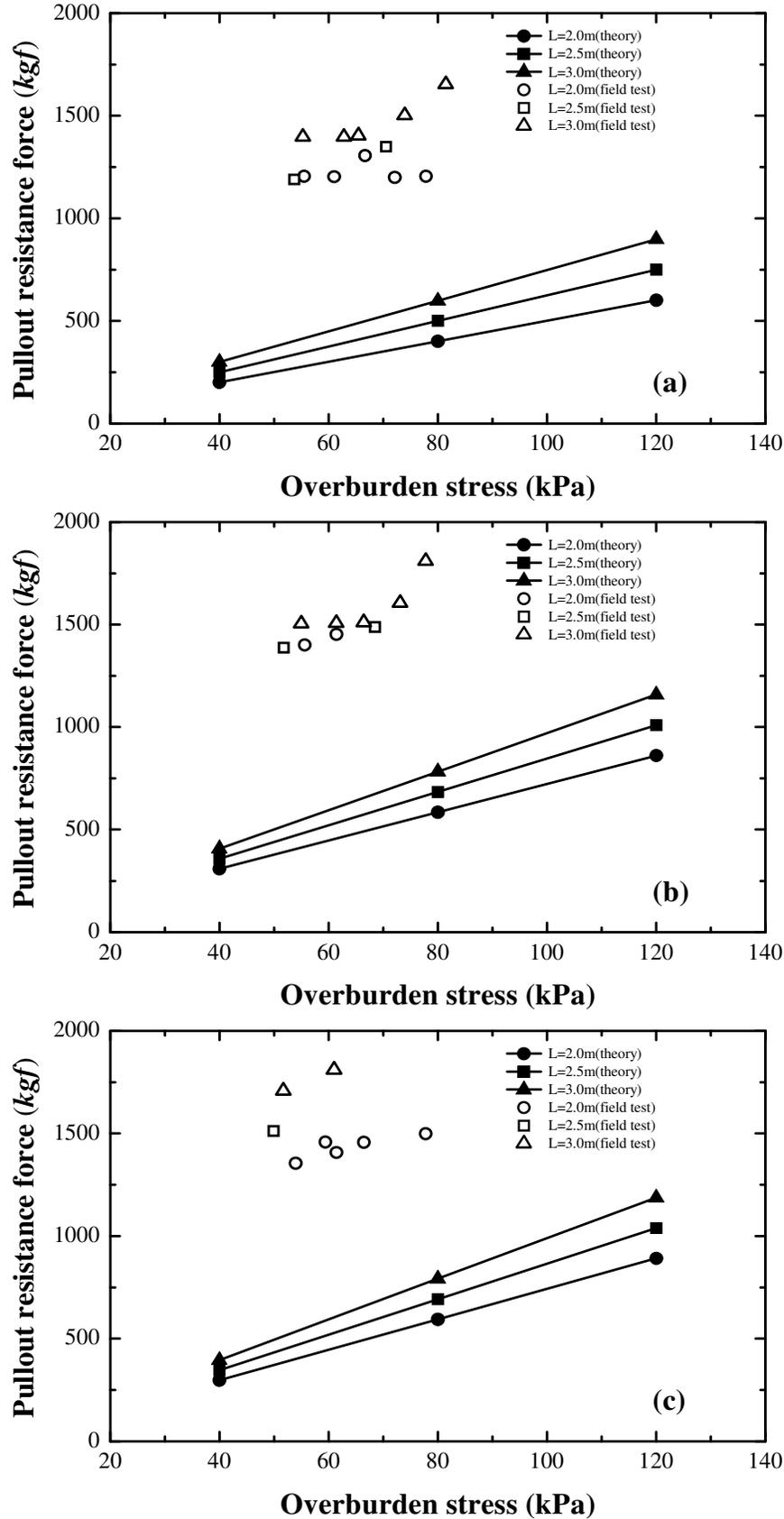
Figure 10. Comparison between *in-situ* pullout test and theoretical computation: (a) Chain, (b) Chain with transverse steel bar and (c) Chain with L-type angle.
