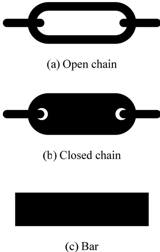
Figure 4. Shapes of various reinforcements.
