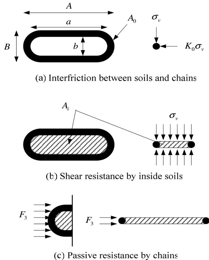
**Figure 1.** Pullout resistance factors of embedded chain in soils (Inoue et al., 1996).
