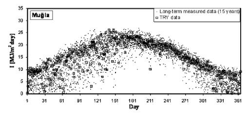
**Figure 3.** Annual variation of long-term measured daily global solar radiation for Muğla and comparison with the generated typical solar radiation  $(I_{TRY})$  data.
