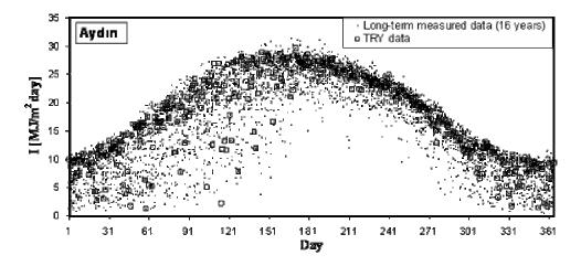
**Figure 2.** Annual variation of long-term measured daily global solar radiation for Aydın and comparison with the generated typical solar radiation  $(I_{TRY})$  data.
