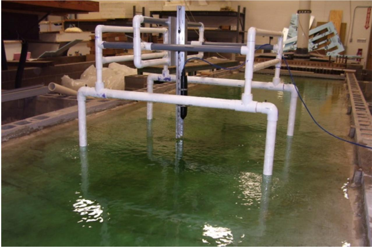
**Figure 1.** ADV, frame and the flow channel.
