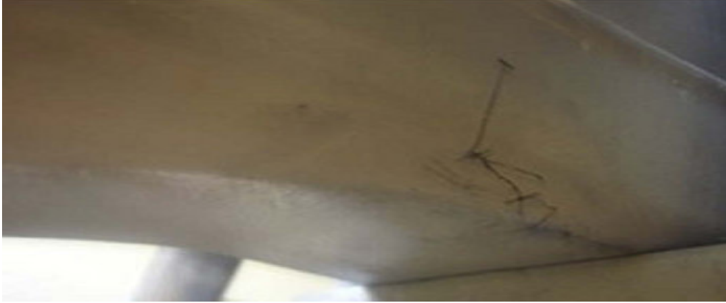
Figure 5. Fatigue failure of a test sample.
