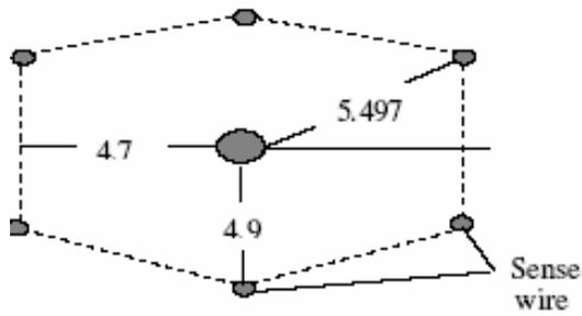
**Figure 1.** The geometry of the ITC drift cell (All dimensions are millimeters).
