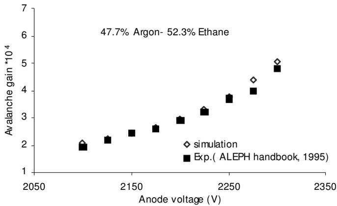
**Figure 2.** The calculated gas gain as a function of anode voltage in an Argon-Ethane mixture.
