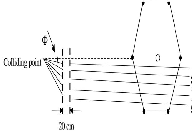
**Figure 3.** Schematic representation of the charged particles passing through the ITC drift cell.
