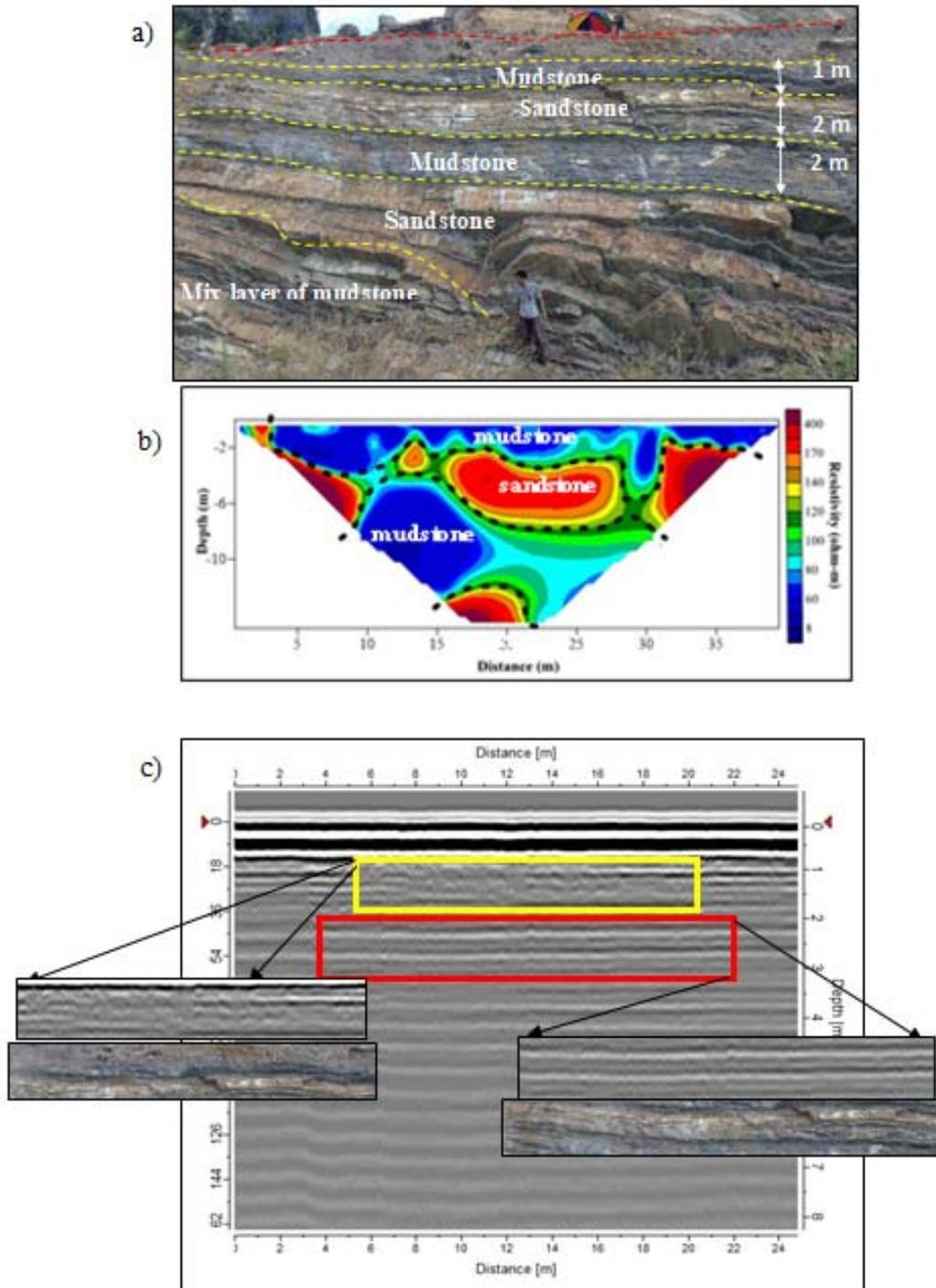
**Figure 5.** (a) Outcrop at Bukit Chondong, (b) Inversion model of 2-D resistivity method shows interbedded of mudstone and sandstone at Bukit Chondong, (c) Layering of mudstone (yellow box) and sandstone (red box) based from the reflective signal.
