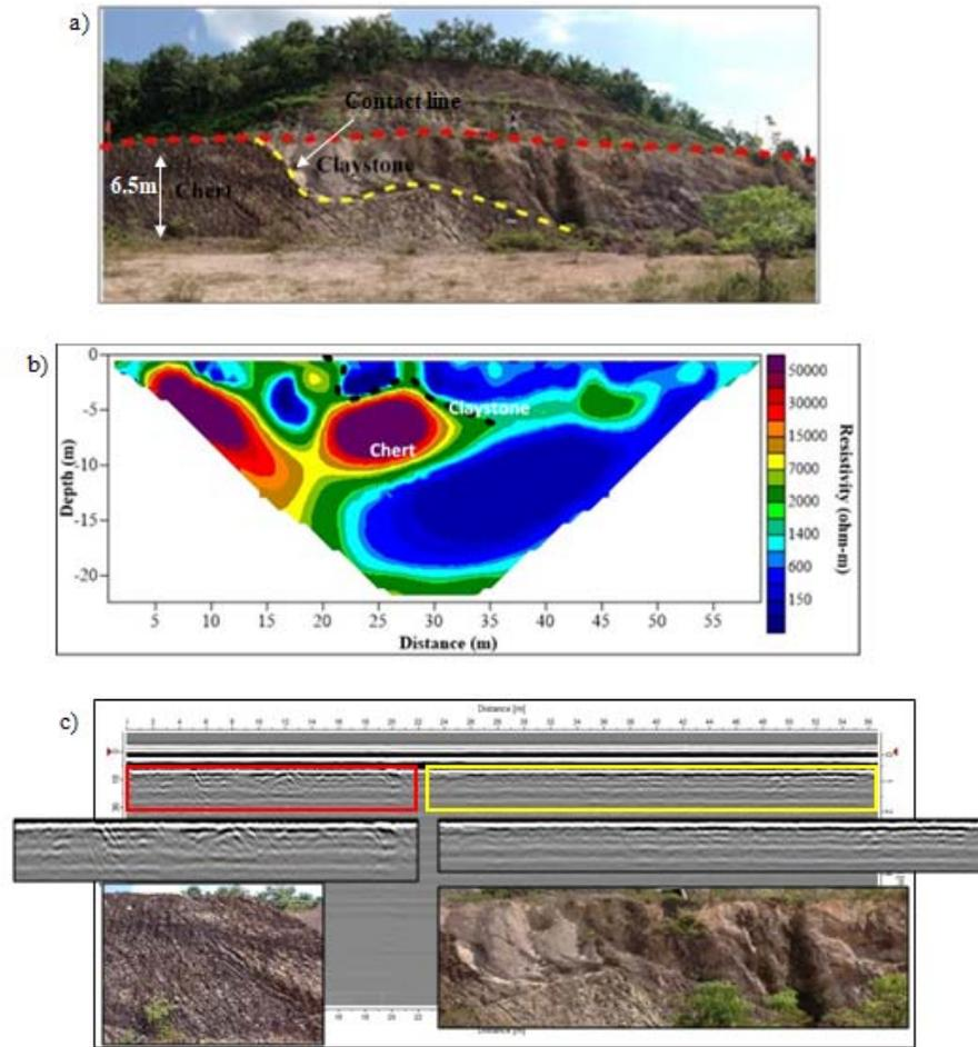
**Figure 7.** (a) Contact between chert and claystone marked with yellow dashes line, (b) Inversion model of 2-D resistivity at Bukit Kukus, (c) Verification of chert (red box) and claystone (yellow box) based from the reflective amplitude contrast.
