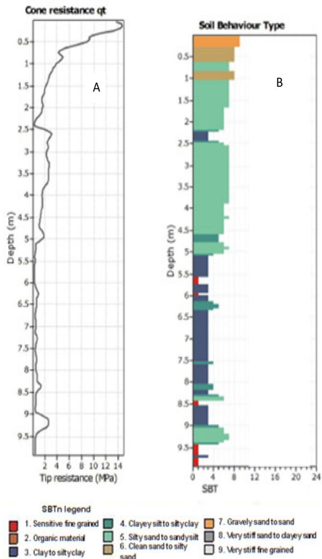
**Figure 1.** Pre-treatment CPT results (A) and soil profile at the project site (B).
