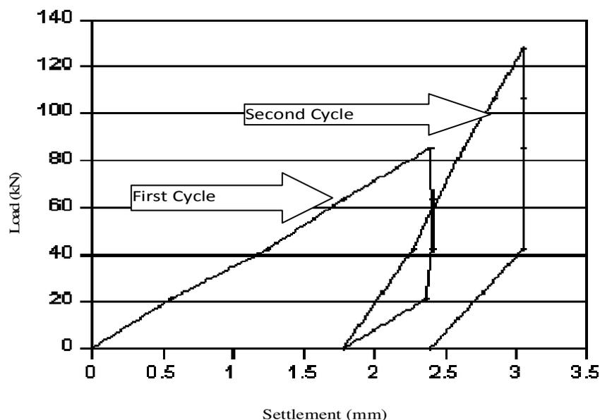
**Figure 4.** Load cycles during the test, under working load.
