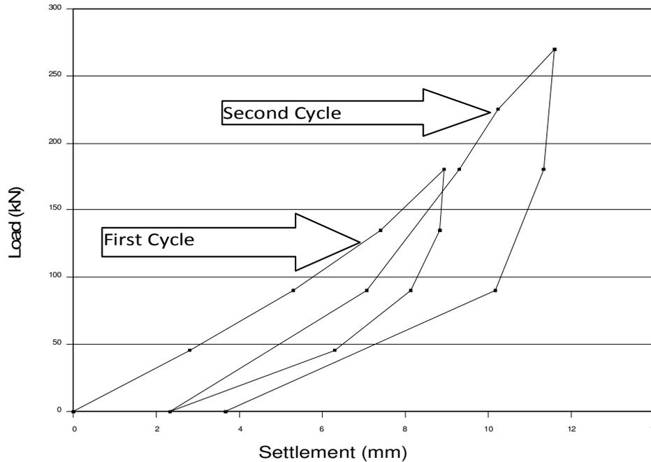
Figure 5. Ultimate load versus settlement.
