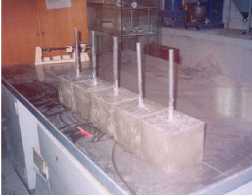
Figure 5. Bond strength specimens after demolding.
