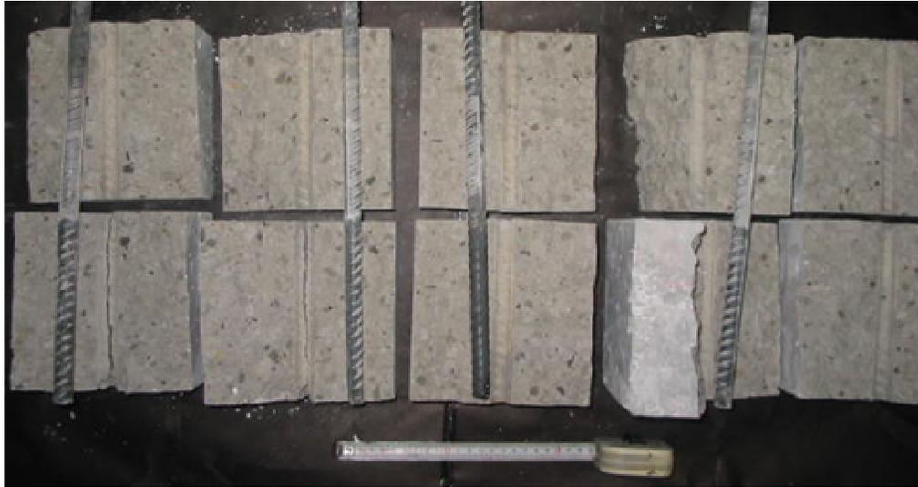
**Figure 21.** Typical failure of SLWAC bond specimens after bond strength testing.
