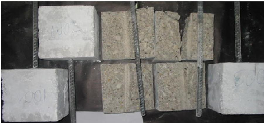
**Figure 20.** Typical failure of NWAC bond specimens after bond strength testing.
