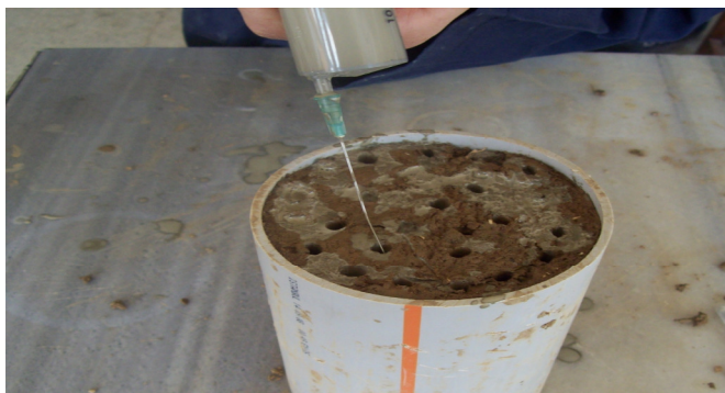
Figure 3. Injection of bentonite + rheocem into soil sample.
