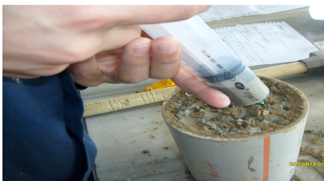
Figure 2. Rheocem injections into soil sample.
