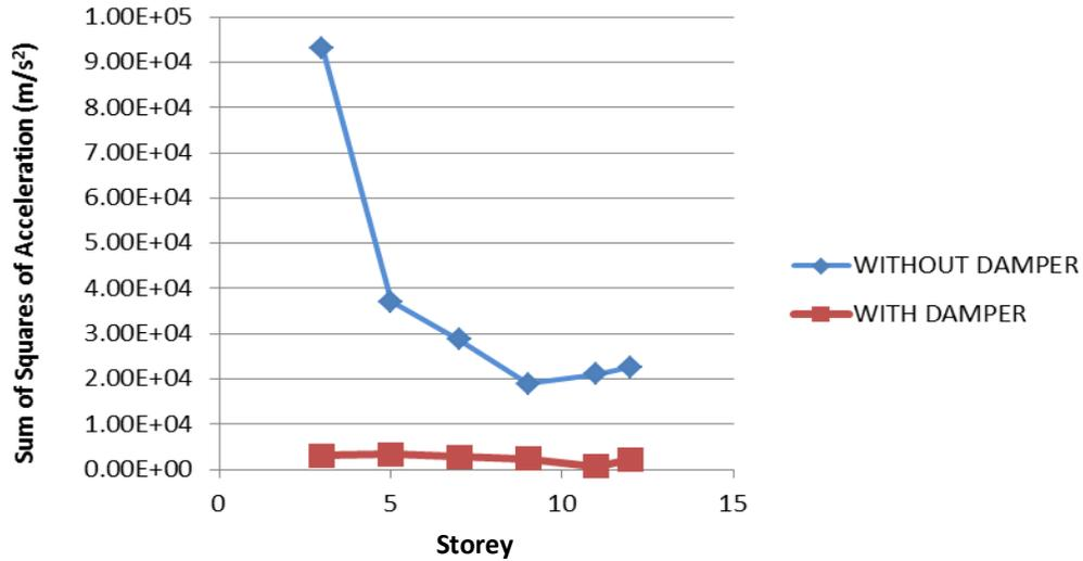
Figure 10. The sum of mean squares of acceleration in structural models.
