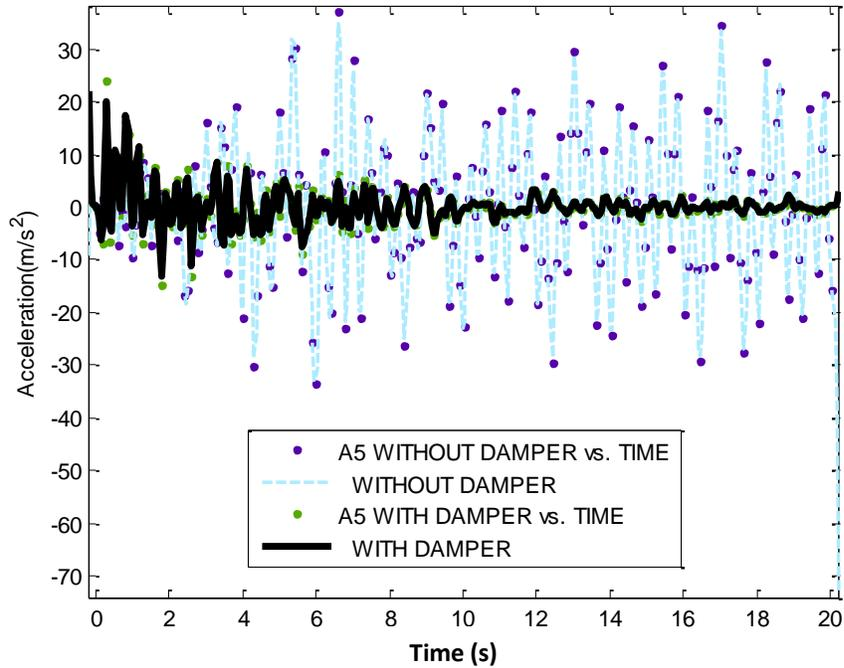
Figure 8. The mean of acceleration in structural models 5 stories with 2 openings.
