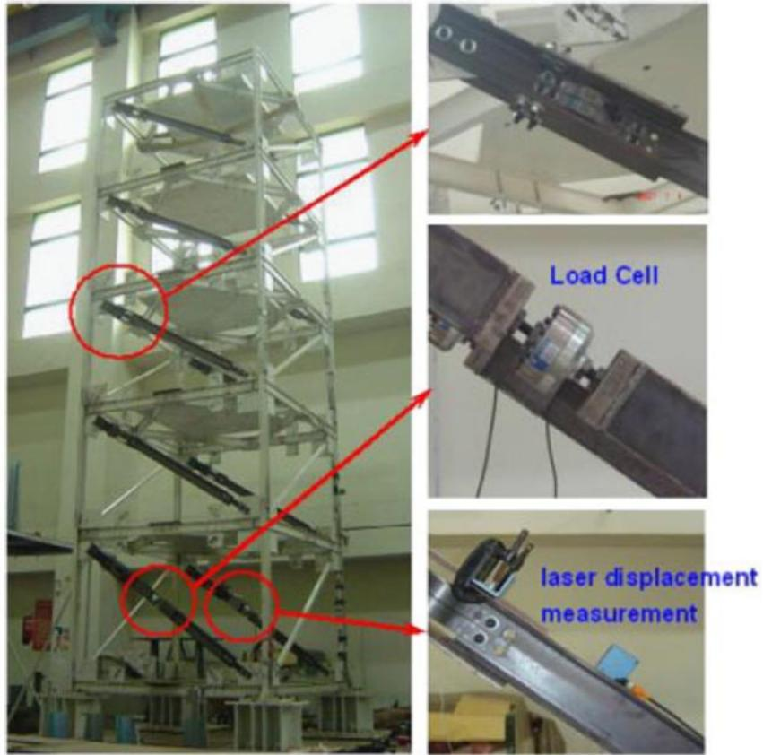
Figure 2. 5 Storey frame on shaking table.
