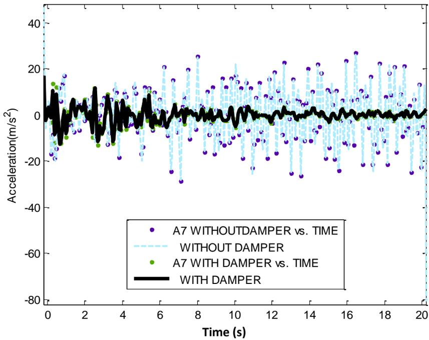
Figure 9. The mean of acceleration in structural models 7 stories with 2 openings.
