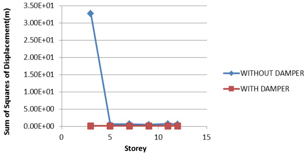
Figure 14. The sum of mean squares of last stories displacement in structural models
