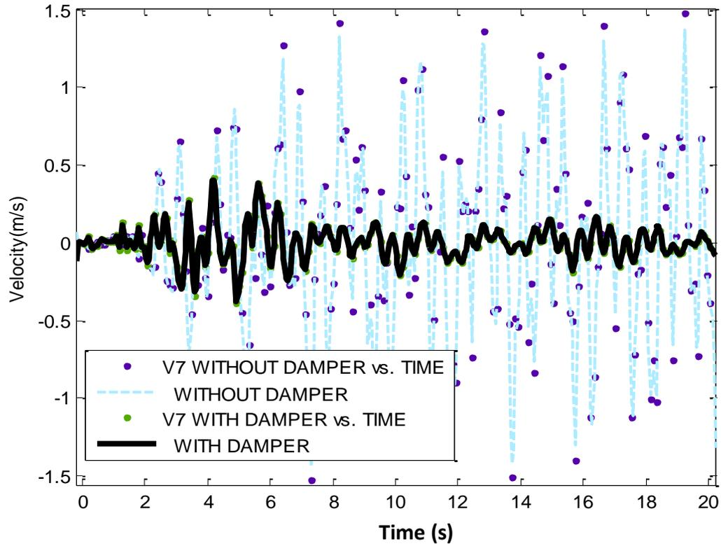
Figure 16. Average velocity of the 7th storey of 7 stories model with two openings.
