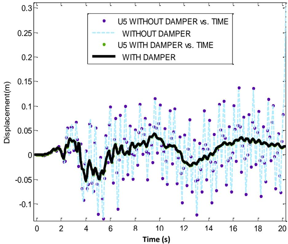
**Figure 12.** Average displacement of the 5th storey of 5 stories model with two openings.
