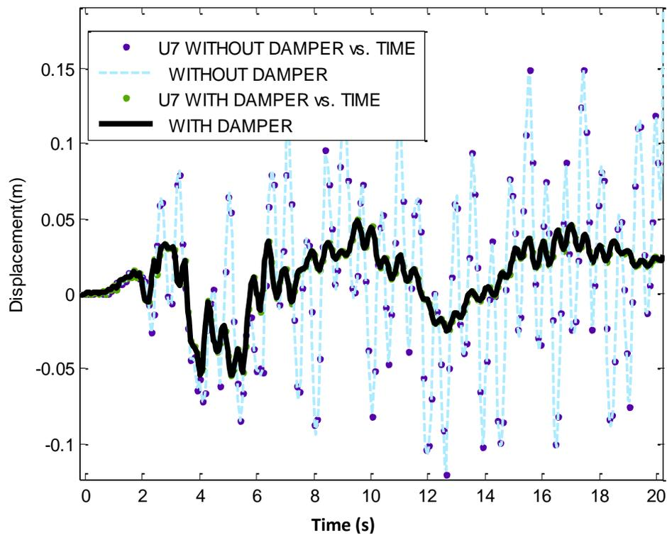
**Figure 13.** Average displacement of the 7th Storey of 7 stories model with two openings.
