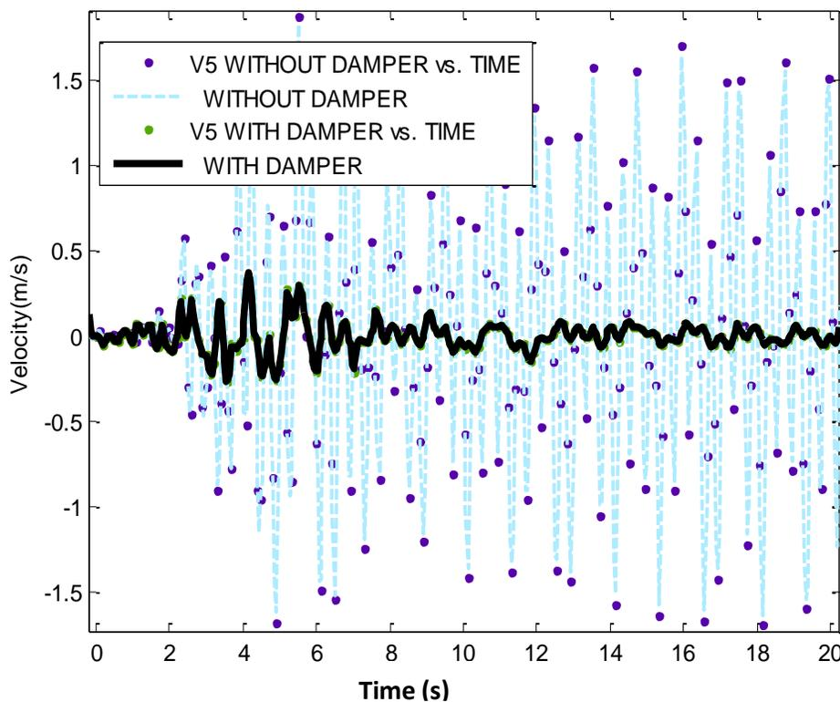
Figure 15. Average velocity of the 5th storey of 5 stories model with two openings.
