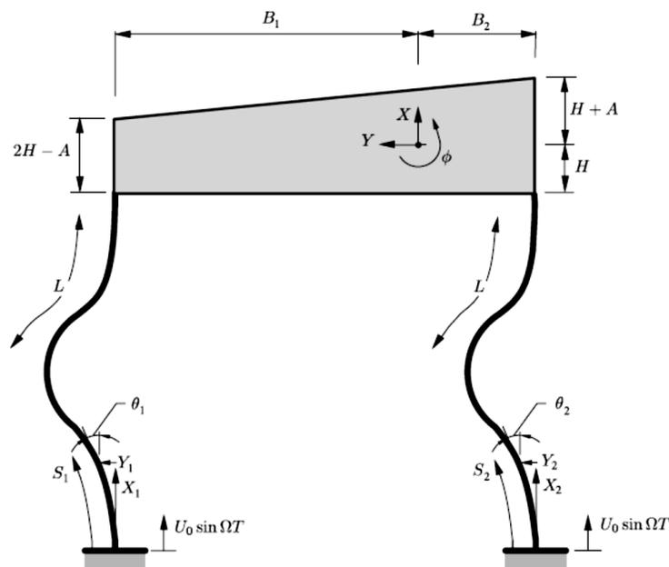
Figure 1. 2D solid diaphragm with pre bent column.
