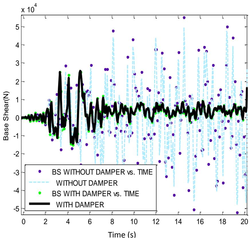
**Figure 5.** The mean of base shear in structural models 7 stories with 2 openings.
