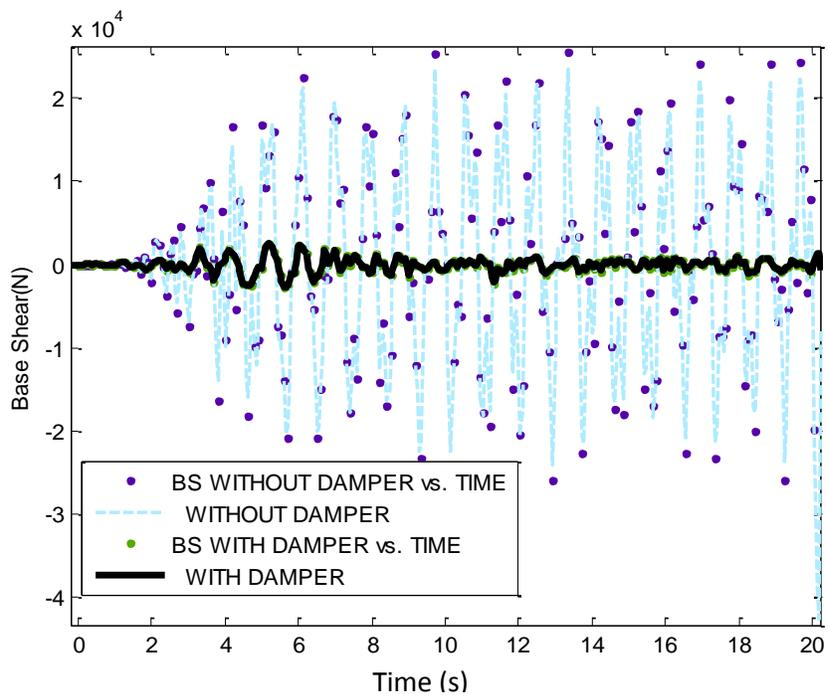
Figure 3. The mean of base shear in structural models 3 stories with 2 openings.
