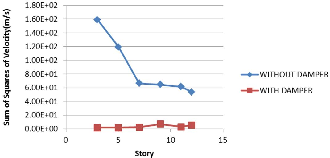
Figure 18. The sum of mean squares of last stories velocity answer in structural models.
