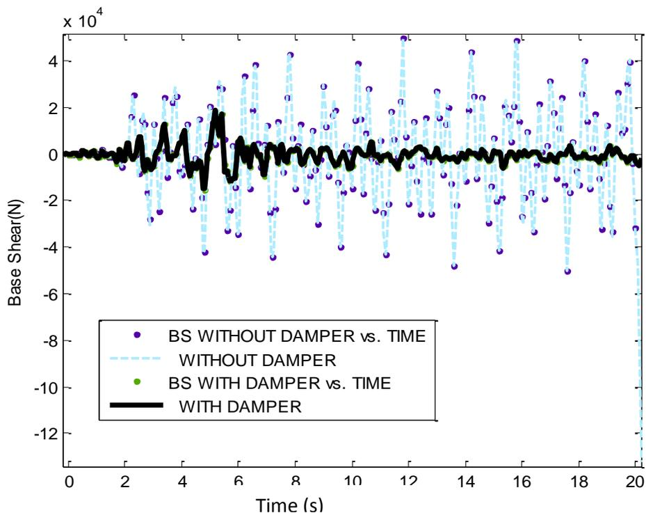
**Figure 4.** The mean of base shear in structural models 5 stories with 2 openings.
