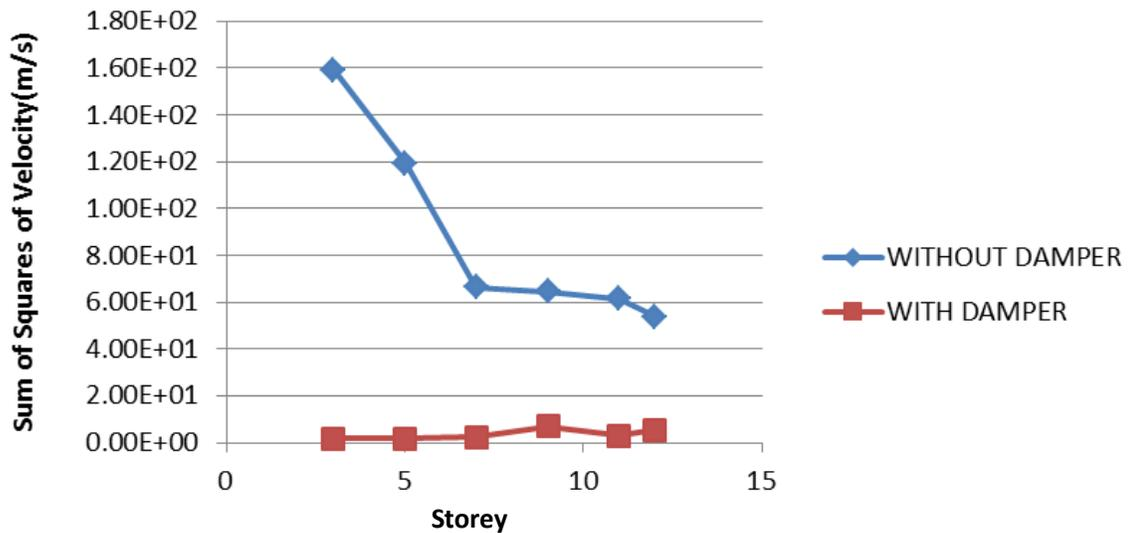
Figure 17. The sum of mean squares of last stories velocity answer in structural models.
