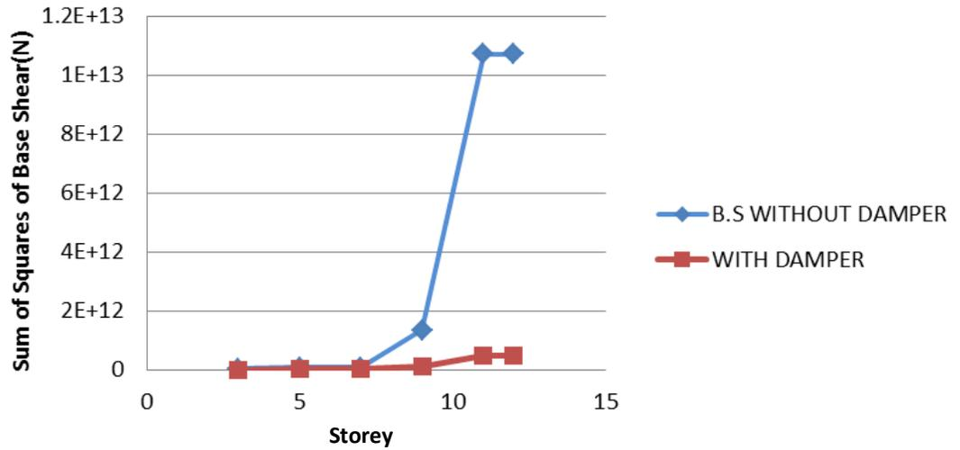
Figure 6. The sum of mean squares of base shear in structural models.
