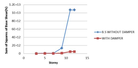
Figure 6. The sum of mean squares of base shear in structural models.
