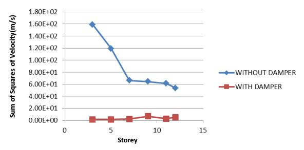
Figure 17. The sum of mean squares of last stories velocity answer in structural models.
