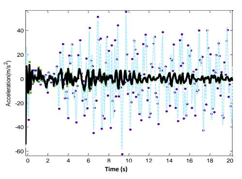
Figure 7. The mean of acceleration in structural models 3 stories with 2 openings.
