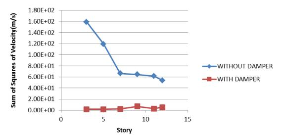
Figure 18. The sum of mean squares of last stories velocity answer in structural models.
