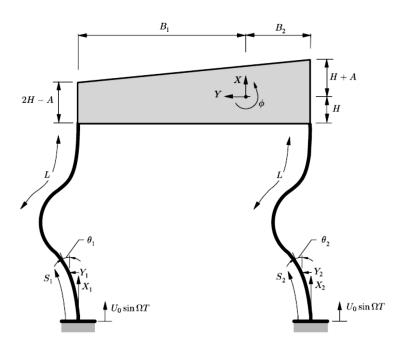
Figure 1. 2D solid diaphragm with pre bent column.
