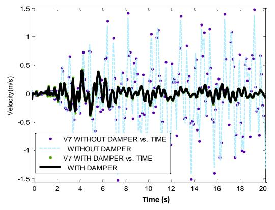
Figure 16. Average velocity of the 7th storey of 7 stories model with two openings.
