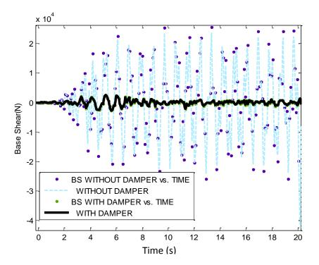
Figure 3. The mean of base shear in structural models 3 stories with 2 openings.
