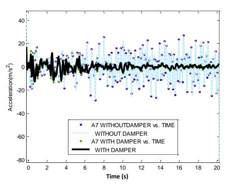
Figure 9. The mean of acceleration in structural models 7 stories with 2 openings.
