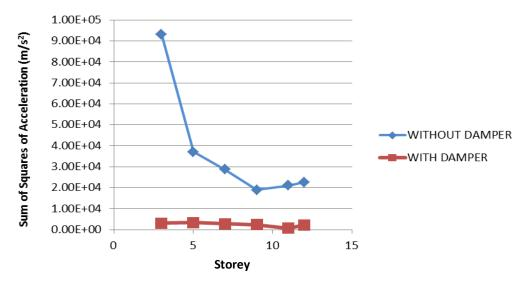
Figure 10. The sum of mean squares of acceleration in structural models.
