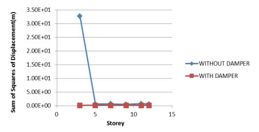
Figure 14. The sum of mean squares of last stories displacement in structural models
