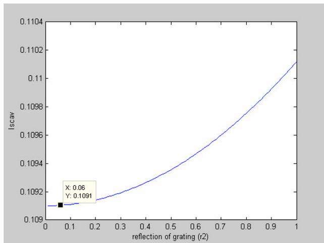
**Figure 5.** Polymer grating reflecting ratio ( $r_2$ ) vs.  $I_{sc}$  under  $r_1 = 0.14$ .
