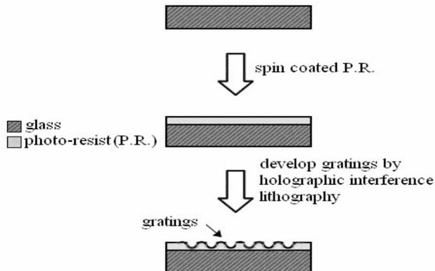
**Figure 2.** Process flow of periodical photo-resist grating.
