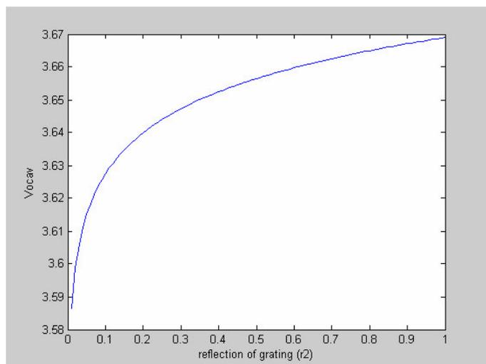
**Figure 6.** Polymer grating reflecting ratio ( $r_2$ ) vs.  $V_{oc}$  under  $r_1 = 0.14$ .
