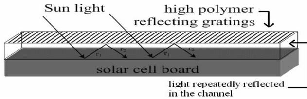
**Figure 1.** Schematic structure of surface gratings and reflecting ratios on the solar cell.
