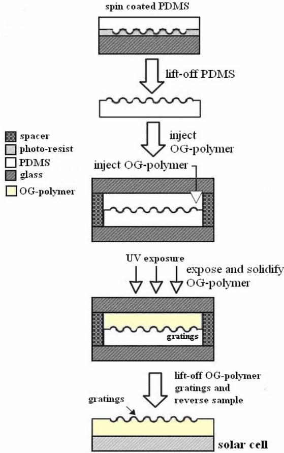
**Figure 3.** Process flow of transferring polymer gratings to reprint on the solar cell.
