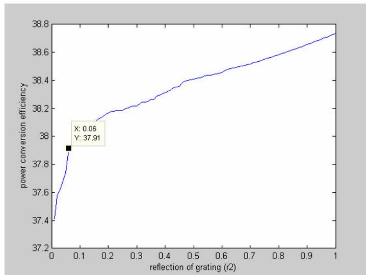
**Figure 7.** Polymer grating reflecting ratio ( $r_2$ ) vs. power conversion efficiency ( $\eta\%$ ) under  $r_1 = 0.14$ .
