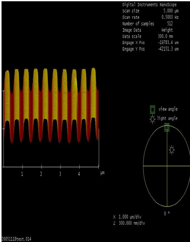
**Figure 4.** Surface reflecting gratings under AFM measurement.
