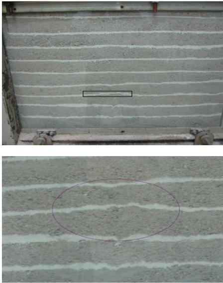
**Figure 3.** Failure mechanism in dense sand at embedment ratio,  $L/D = 4$ .
