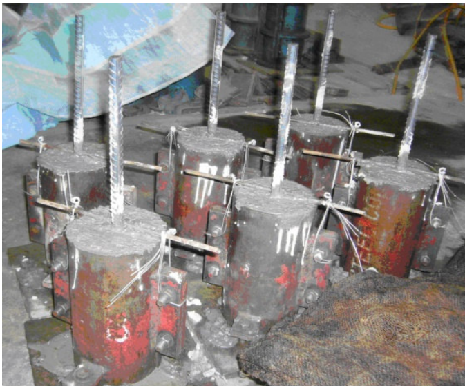
Figure 3. Preparation of pull-out specimens.
