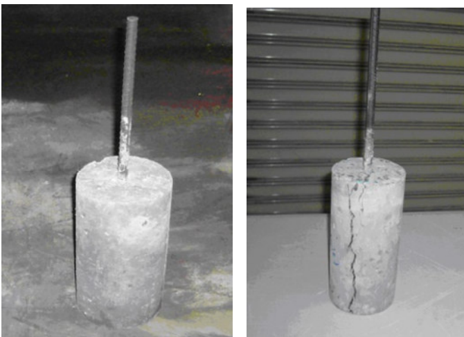
Figure 7. Pull-out failure of specimen. (a) Before test. (b) OPKSC after failure.
