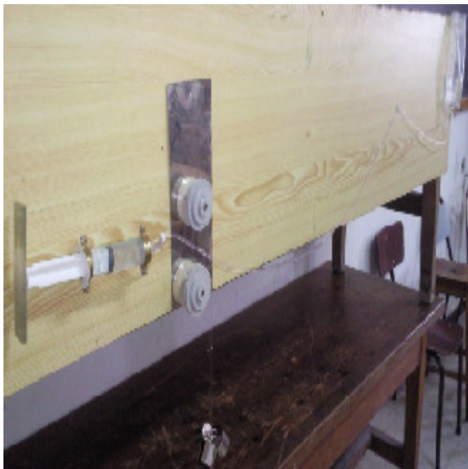
Figure 3. Experimental assembly for the determination of friction in the syringe.
