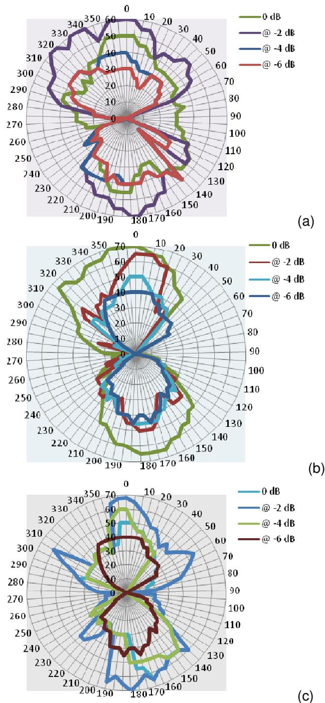
**Figure 4.** (a) Co-polarization radiation of plastic tags in free environment. (b) Co-polarization radiation of plastic tags in metallic environment and (c) Cross polarization radiation of plastic tags in free environment.
