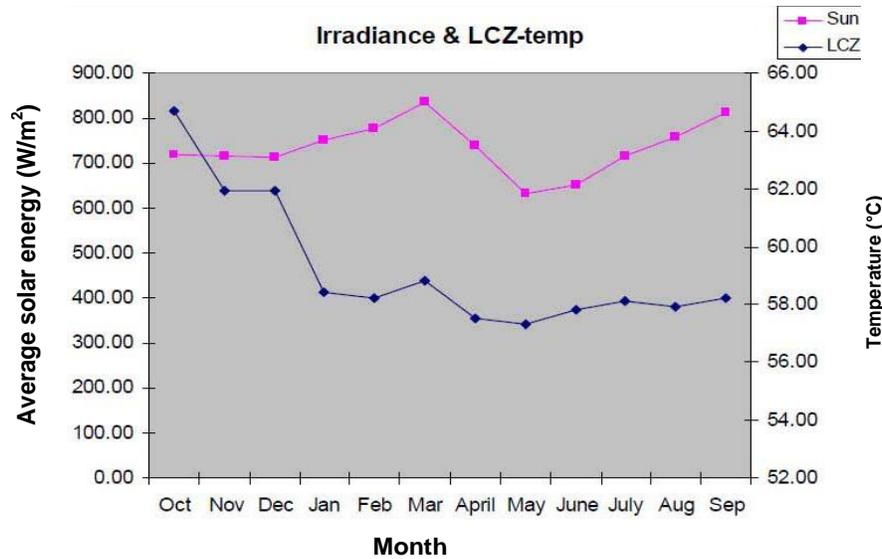
Figure 13. The temperature variation of LCZ and the monthly average solar energy.
