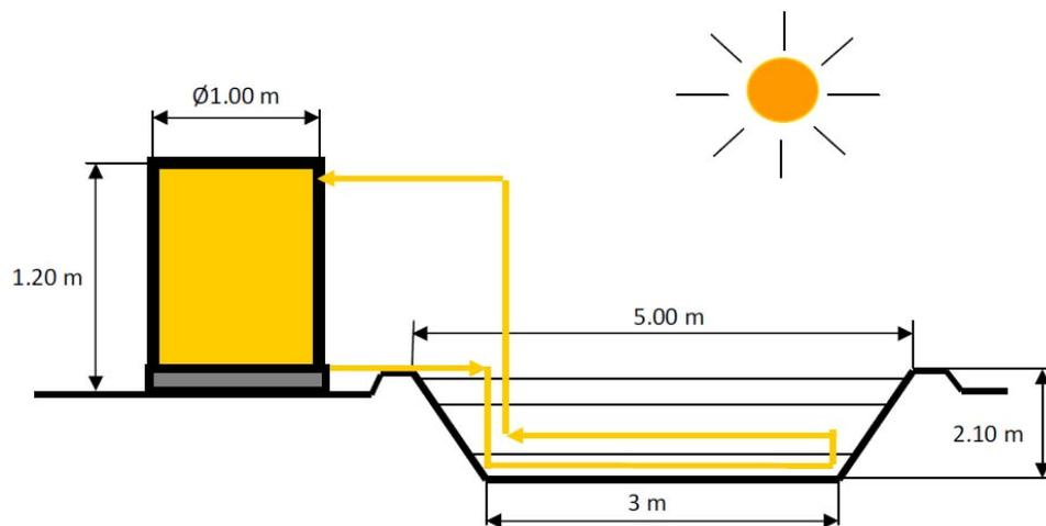
Figure 4. The saline water preheating system.
