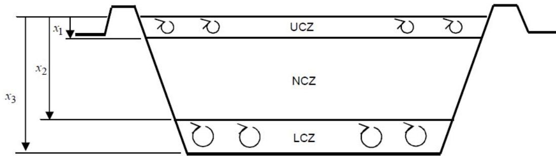
Figure 1. Schematic of a solar pond (Huanmin et al., 2004).
