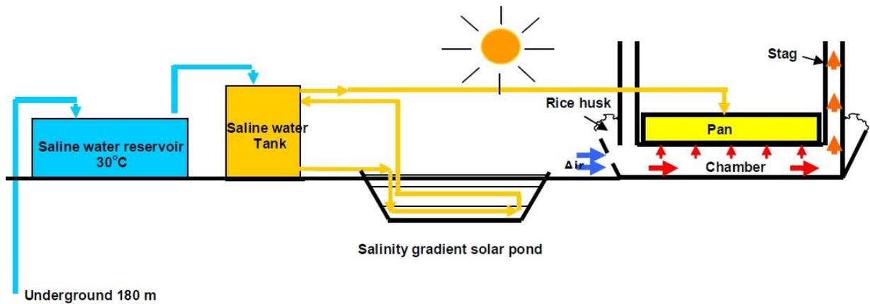
Figure 3. Lining scheme of saline water preheating system.
