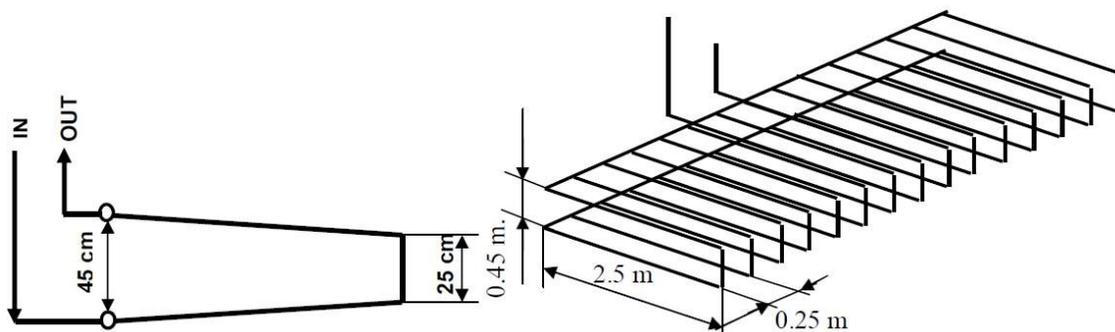
Figure 5. The thermosyphonic coil.
