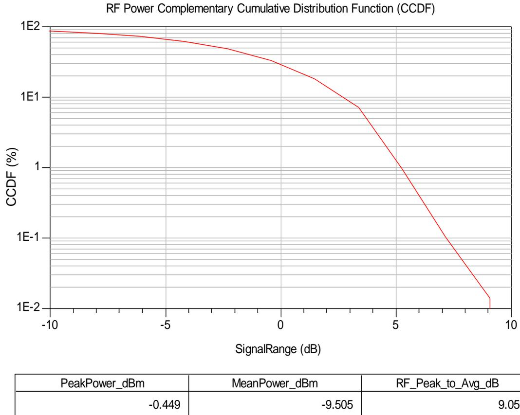
Figure 1. Transmitter CCDF downlink and uplink.
