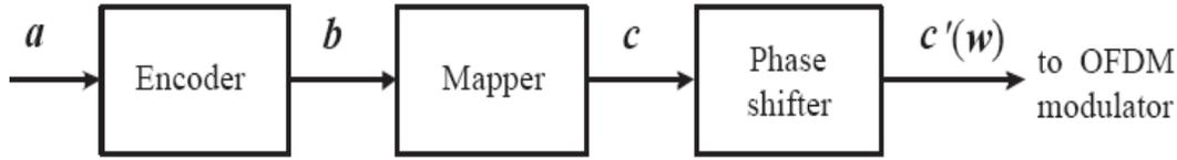
**Figure 10.** Coding and phase rotation for simultaneous error control and PAPR reduction.
