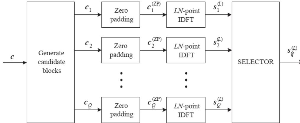
Figure 8. Block diagram of the SLM technique.
