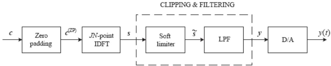
Figure 7. Clipping and filtering operations on the oversampled OFDM signal.
