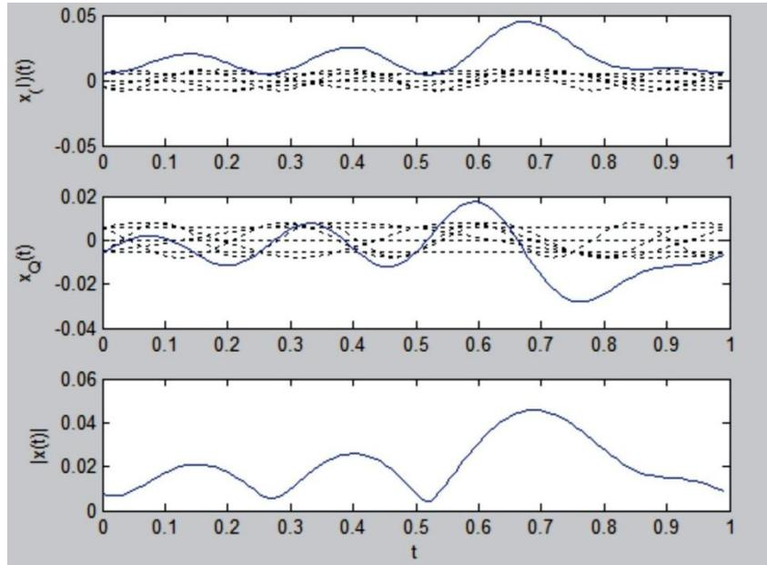
Figure 3. Individual time domain QPSK modulated subcarriers.
