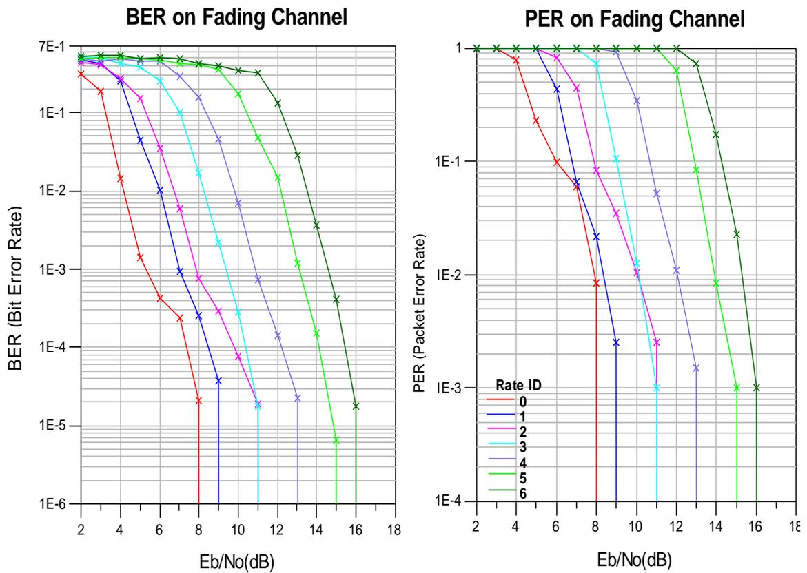
Figure 6. Uplink BER & PER on a fading channel.
