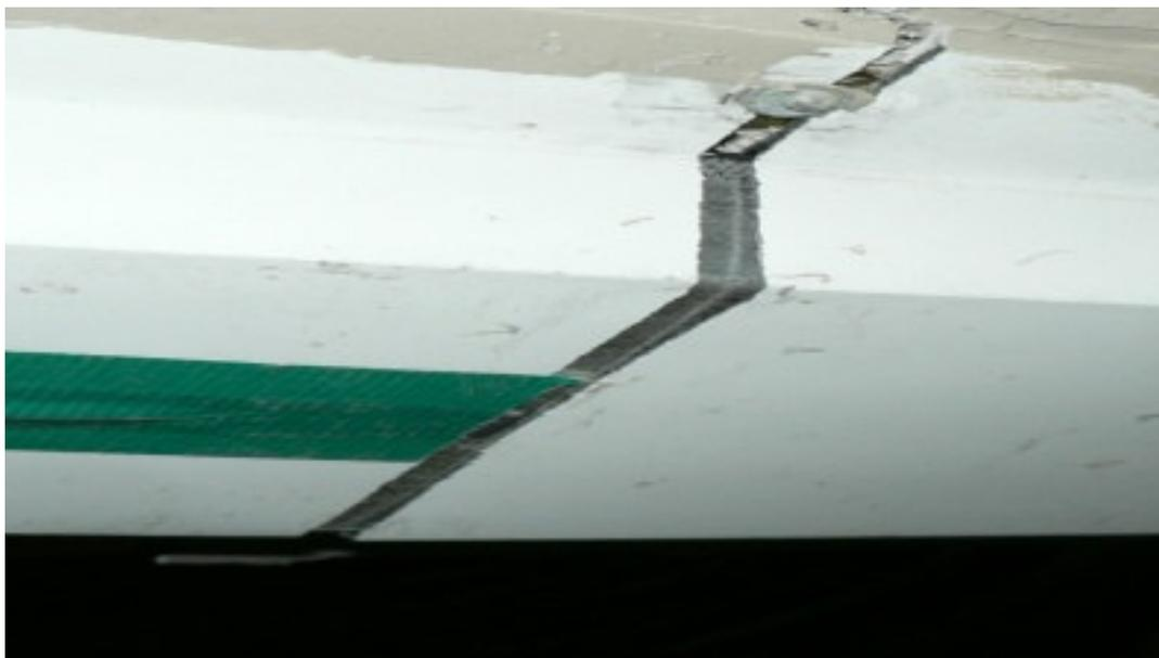
**Figure 10.** Fracture failure of composite-beam.
