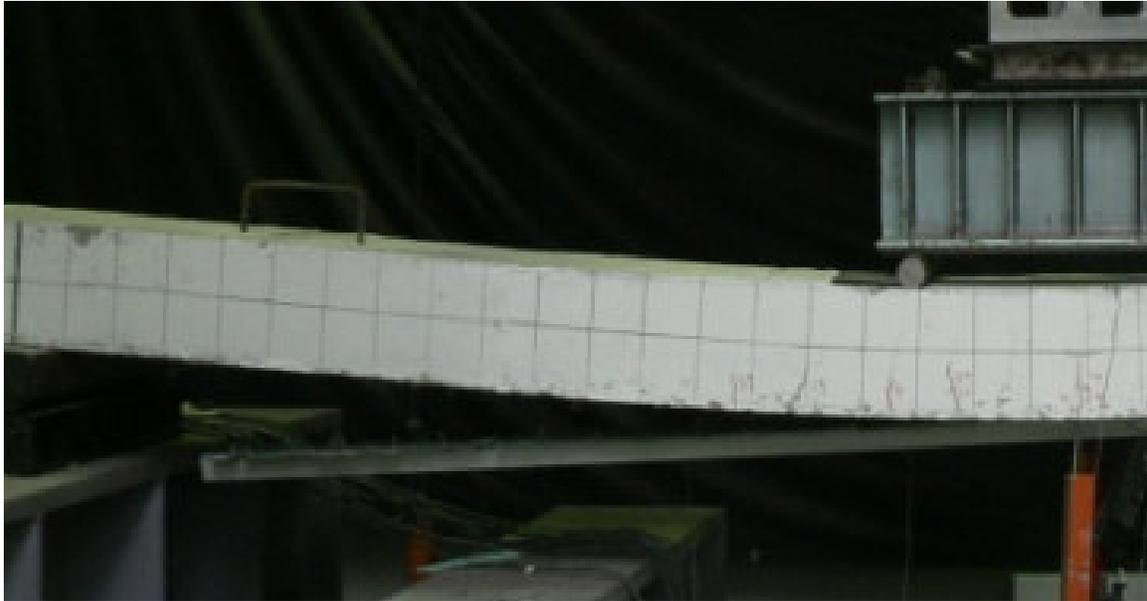
**Figure 9.** Debonding failure of composite-beam.
