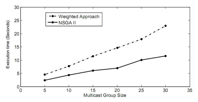
Figure 10. Effect of multicast group on the convergence time on 100-node network.
