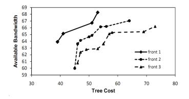
Figure 5. Initial Pareto fronts for 15-node Bellcore network.
