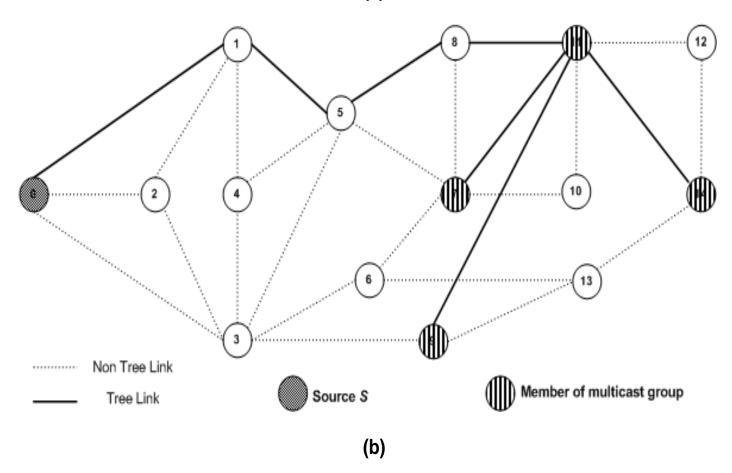
Figure 7. Representation of optimal compromise solution and multicast tree: (a) encoded best compromise solution and tree, (b) best compromise optimal tree on network topology.
