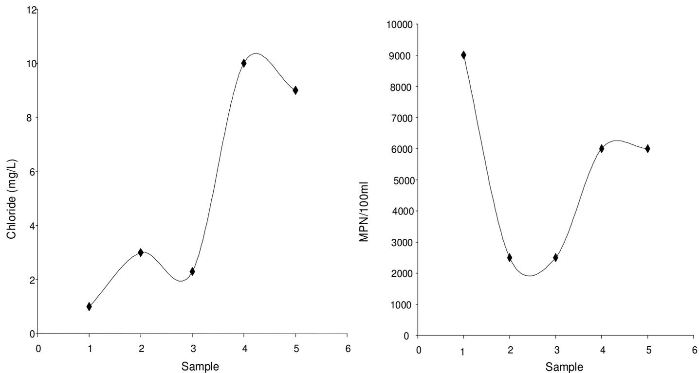
Figure 5. Characteristics of well water used as control for the solar disinfection.
