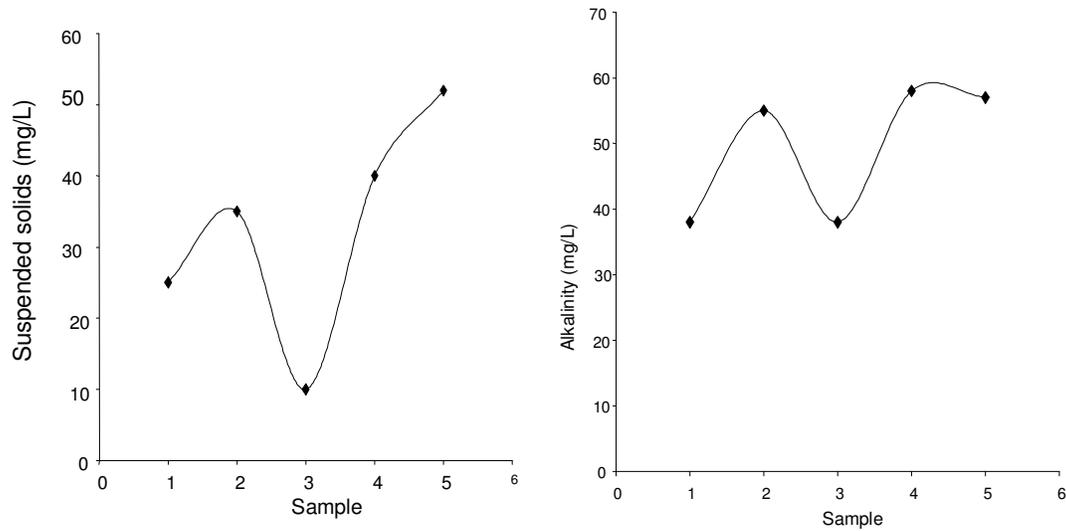
**Figure 3.** Characteristics of well water used as control for the solar disinfection process.
