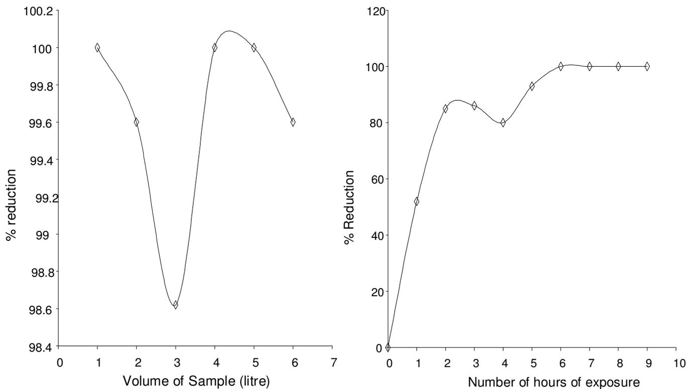
Figure 6 (a). Effect of volume of water on efficacy of solar disinfection. (b) Effect of number of hours of exposure to solar radiation.
