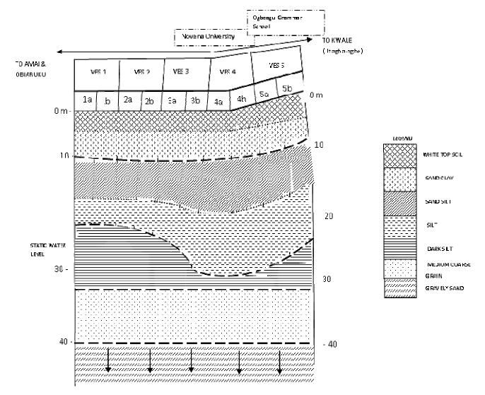
Figure 8. Geoelectric section of Ogume, Delta State.
