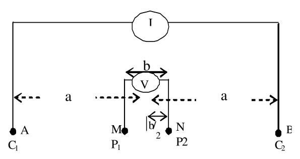
Figure 2. Schlumberger field electrode configuration.
