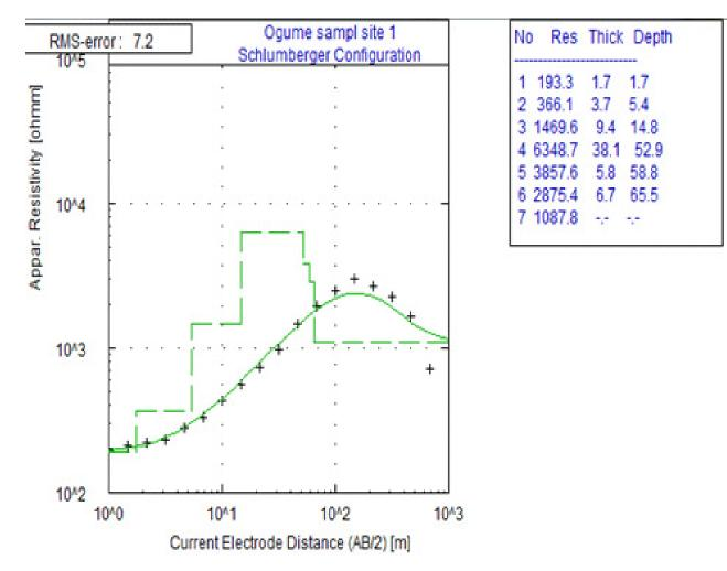
Figure 3. Sample resist graph for site 1 in Ogume.
